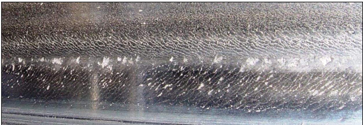
Figure 1. Wheel Tread Surface with RCF Cracks
