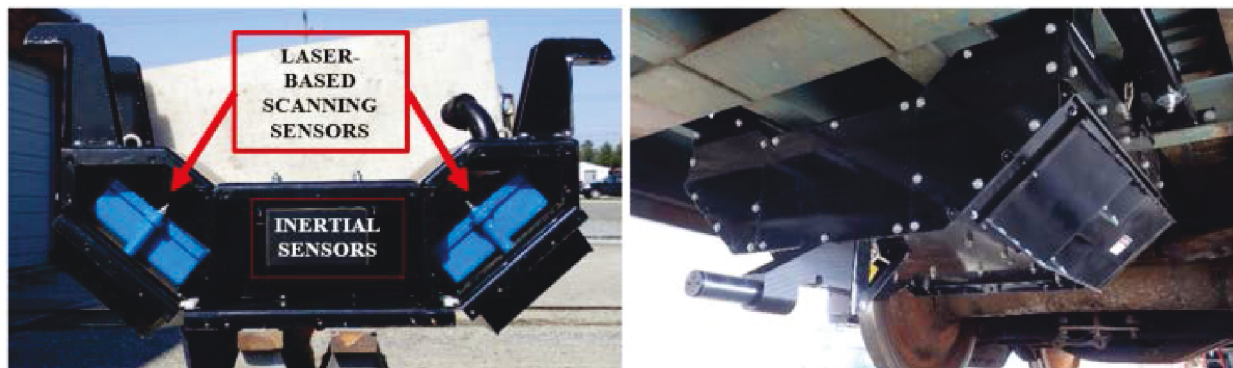
Figure 45: DOTX 225 Geometry Measurement Beam
