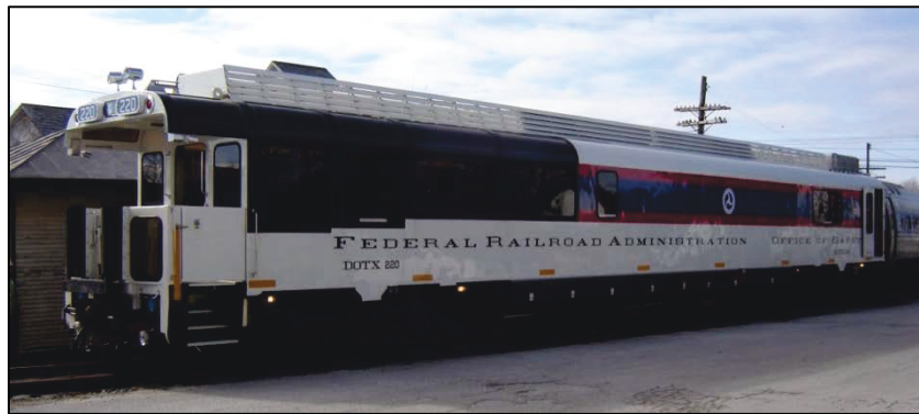
Figure 21: ATIP Manned Geometry Inspection Vehicle—DOTX 220
