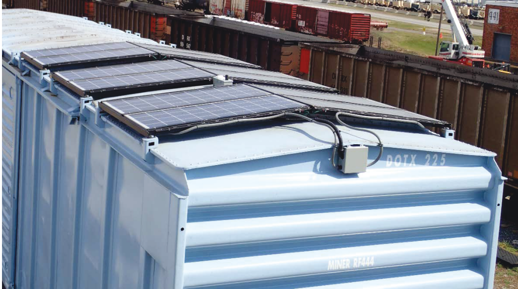
Figure 49: Roof-Mounted Equipment on DOTX 225
