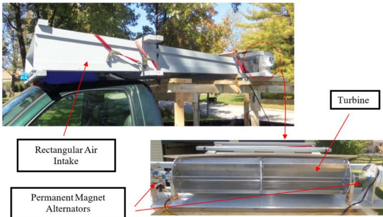
Figure 39: Horizontal Turbine and Rectangular Air Intake Configuration Prototype
