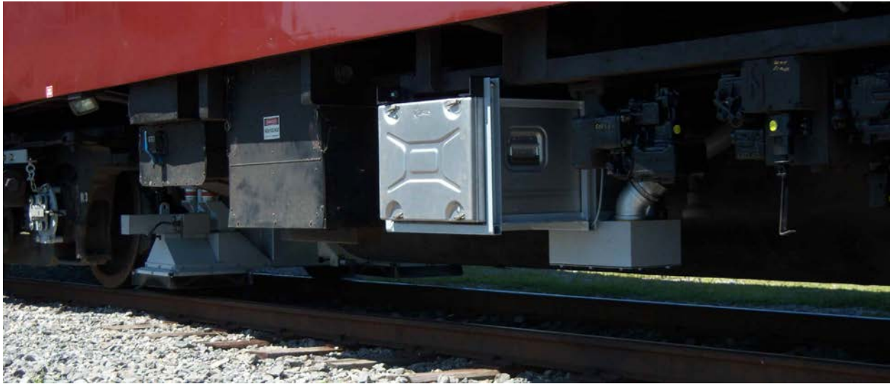
Figure 25: ATGMS Electronics Box on DOTX 221
