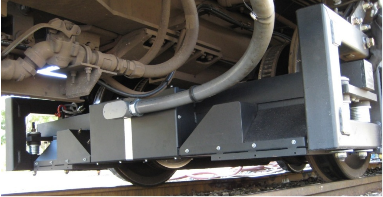
Figure 13: Stage 1 ATGMS Measurement Beam on Amtrak Car 39000
