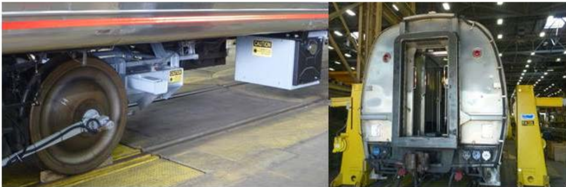
Figure 38: Stage 3 Carbody-Mounted ATGMS Installation, Amtrak's 82602
