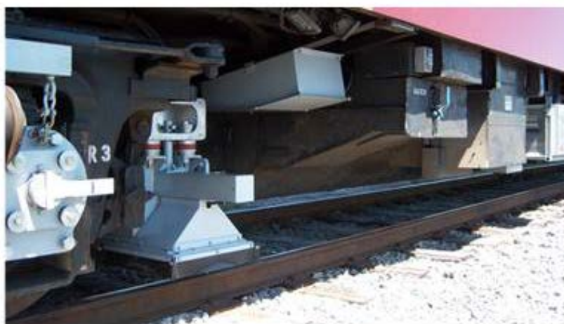
Figure 24: ATGMS Installation on DOTX 221
