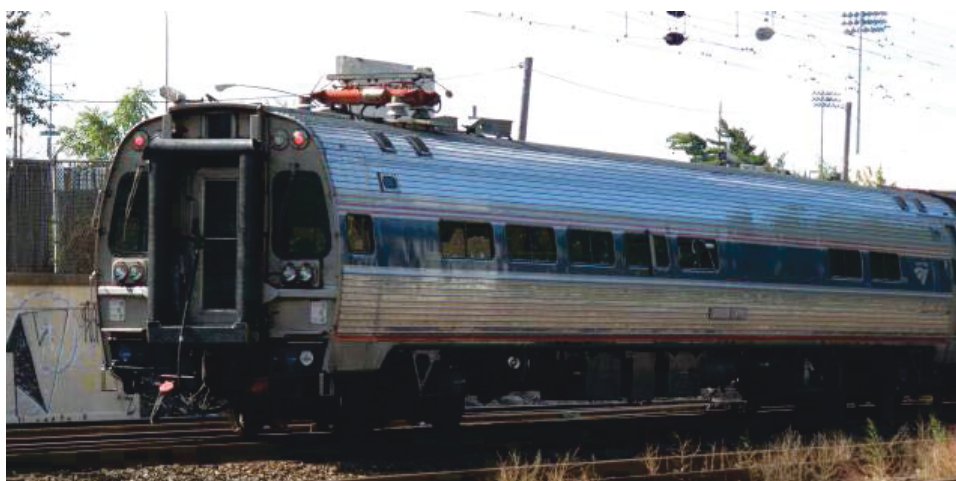
Figure 29: Amtrak's Manned Inspection Vehicle, Amtrak 10002
