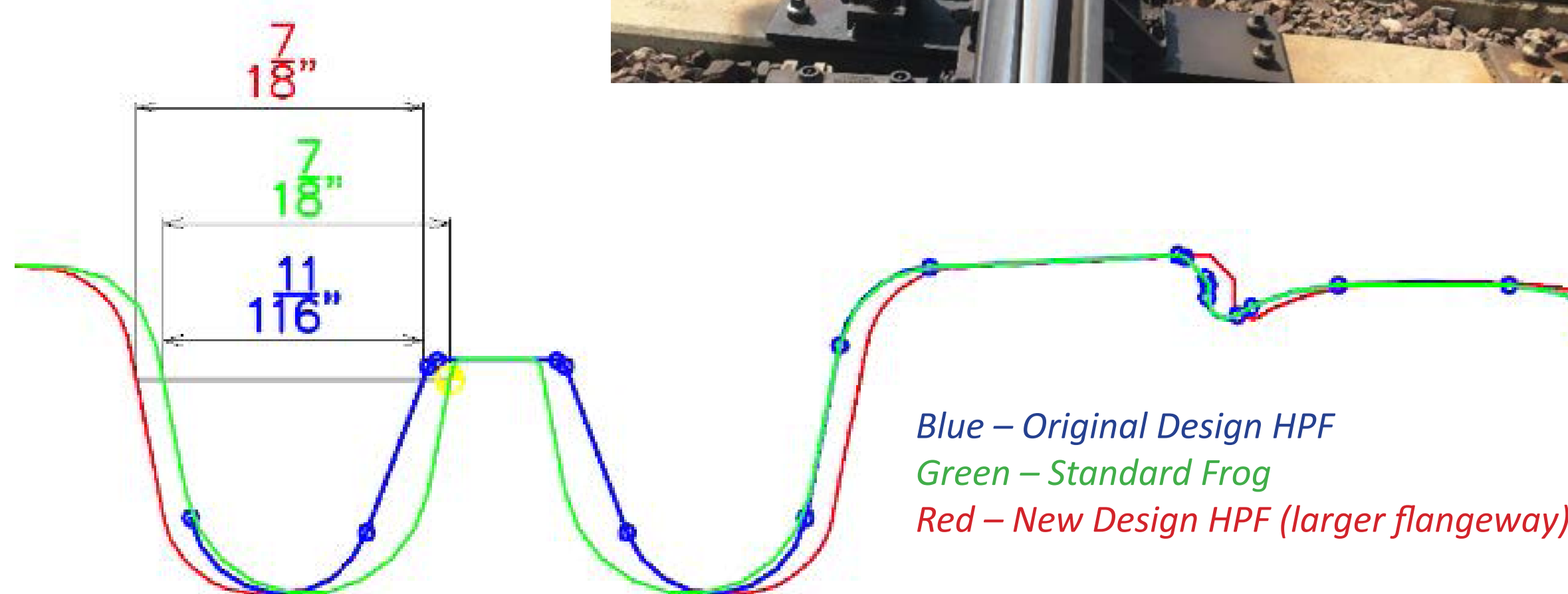
Heavy-Point Frog (HPF) Performance Evaluation – Base Case and Modified Frogs
