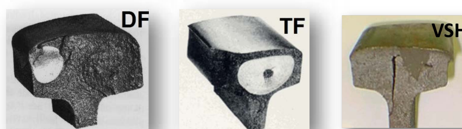
Examples of rail flaws relevant to safety (Left to right: Detail Fracture, Transverse Fissure, and Vertical Split Head)
