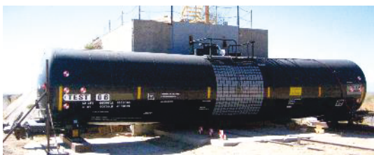
Figure 1. Pre-test Photo of DOT-117
