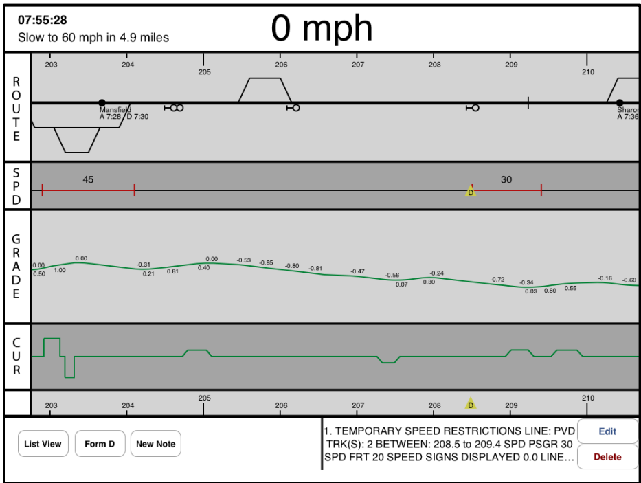
Figure 7. Once the Form D is selected, a yellow triangle icon with the letter “D” appears at the milepost location of the directive.
