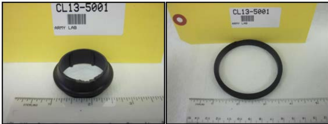
Figure A17. CL13-5001 – Fuel Filter Elastomer Set – II: Sample-1 (Left), Sample-2 (Right)
