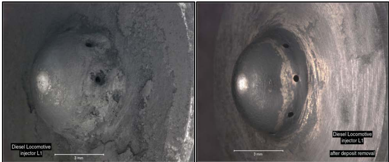
Figure C5. Backscatter Image Showing Fuel Inlet Before and After Deposit Removal
