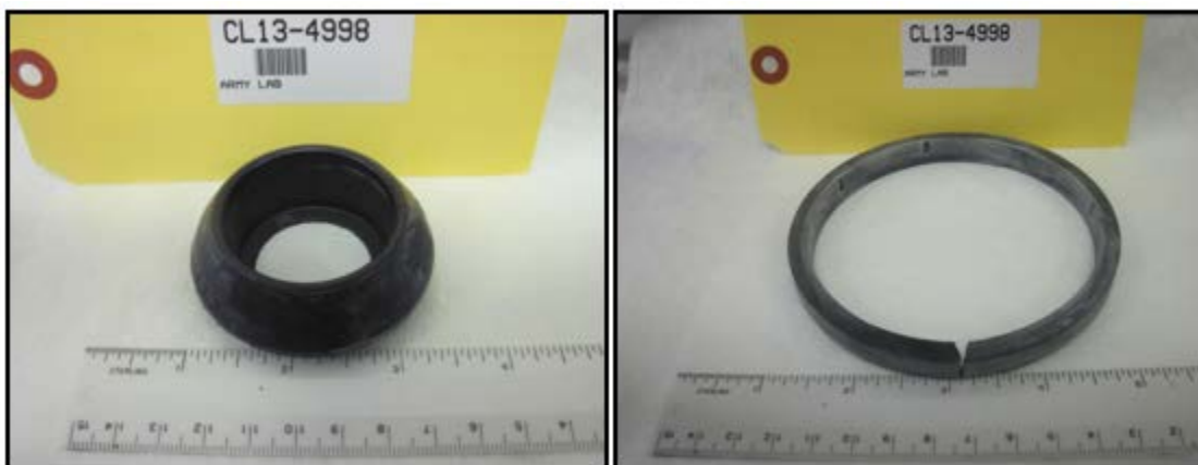
Figure A8. CL13-4998 – Fuel Filter Elastomer Set – I: Sample-1 (Left), Sample-2 (Right)
