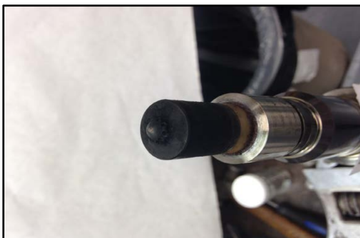
Figure C3. Injector Disassembly Showing Injector Tip
