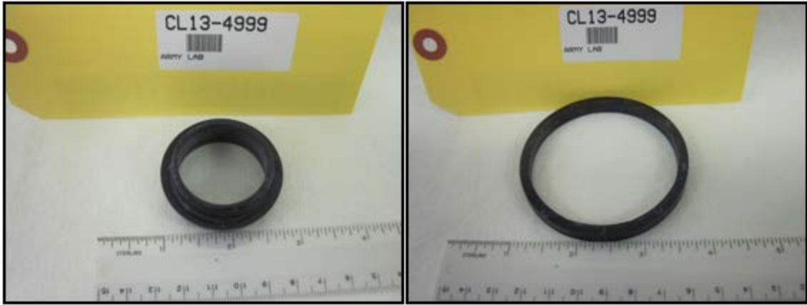
Figure A11. CL13-4999 – Fuel Filter Elastomer Set – I: Sample-1 (Left), Sample-2 (Right)
