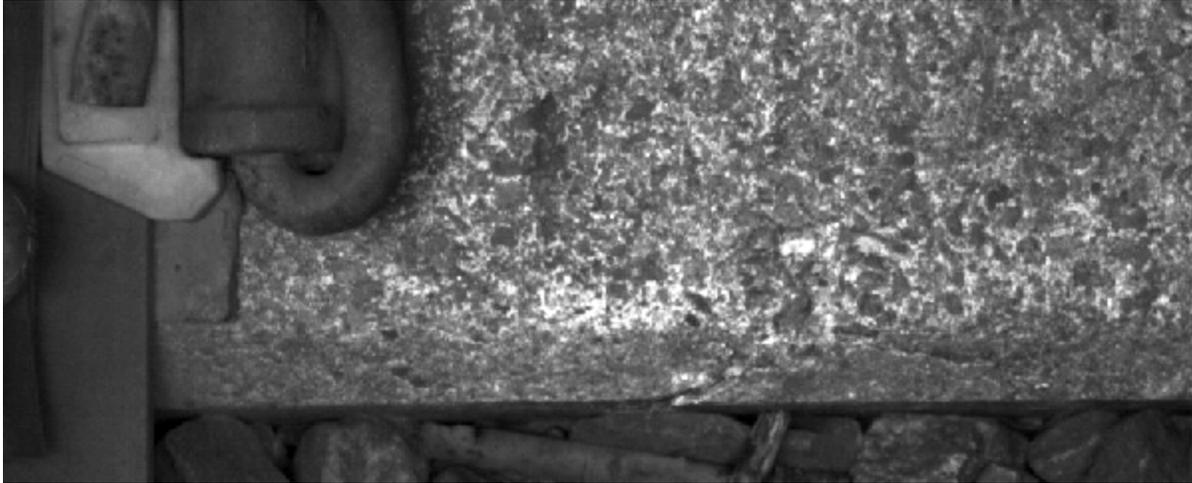
**Figure A-3. Example of a Typical Edge Crack**
