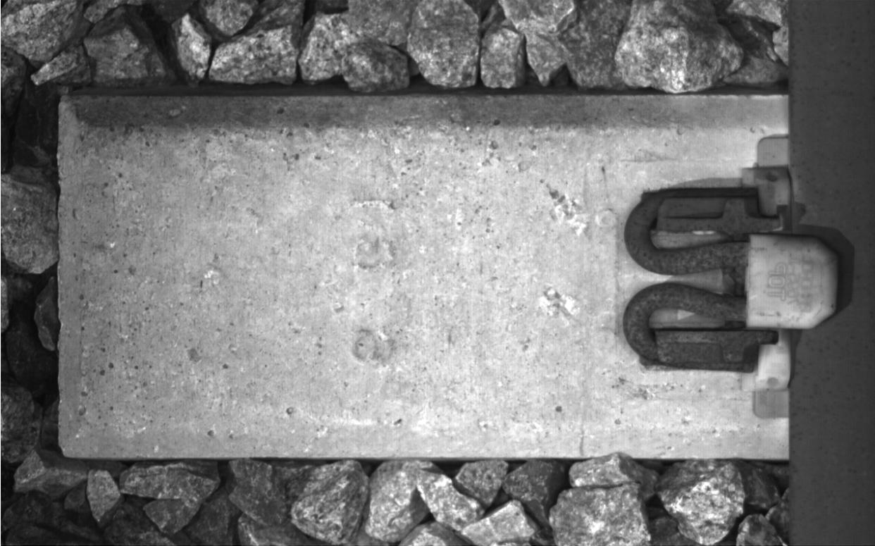
**Figure B-6. Tie Shoulder with Inconsequential Surface Irregularities—Tie Grade = 1**
