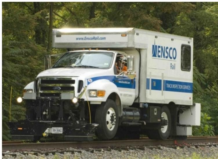
**Figure 2-1. High-Rail Vehicle Used to Collect Track Bed Images**
