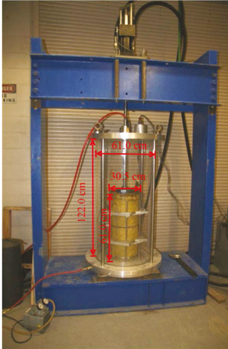
Figure 4.3. Large Scale Triaxial Test Device in the University of Illinois (TX-24)
