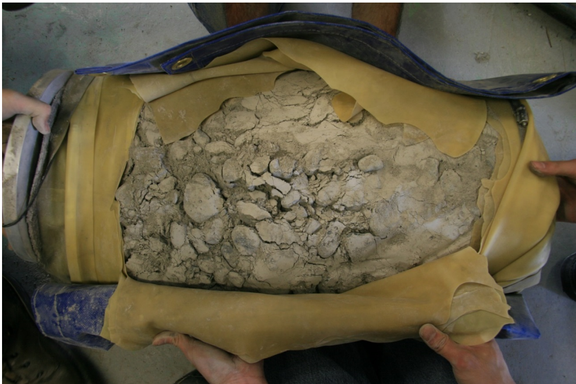
Figure 6.3. Fouled Ballast Specimen (FI=40) After Laboratory Permanent Deformation Testing
