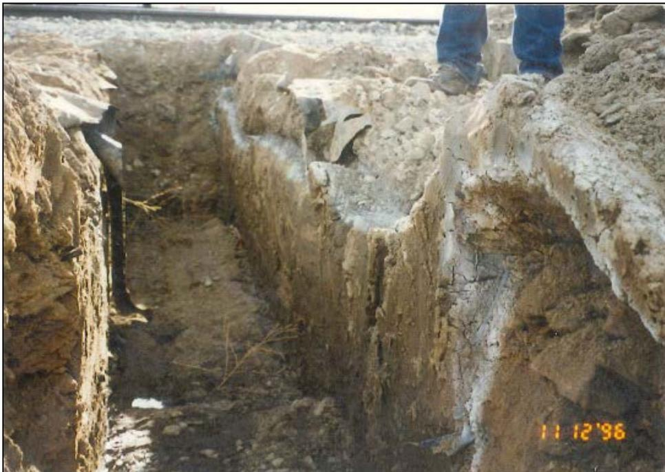
**Figure 7: Cross-Trench for Soil Investigation**
