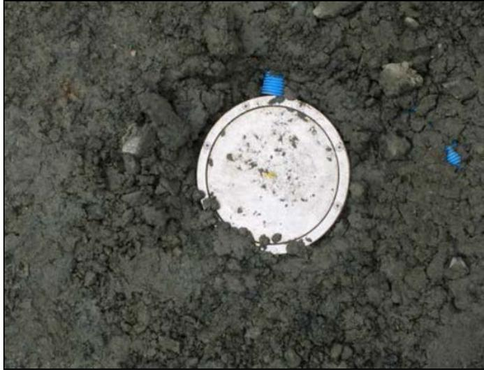
**Figure 31: Pressure Cell Close-Up**
