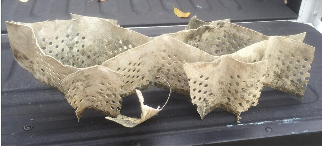
**Figure 66: Side View of the Geocell Sample**
