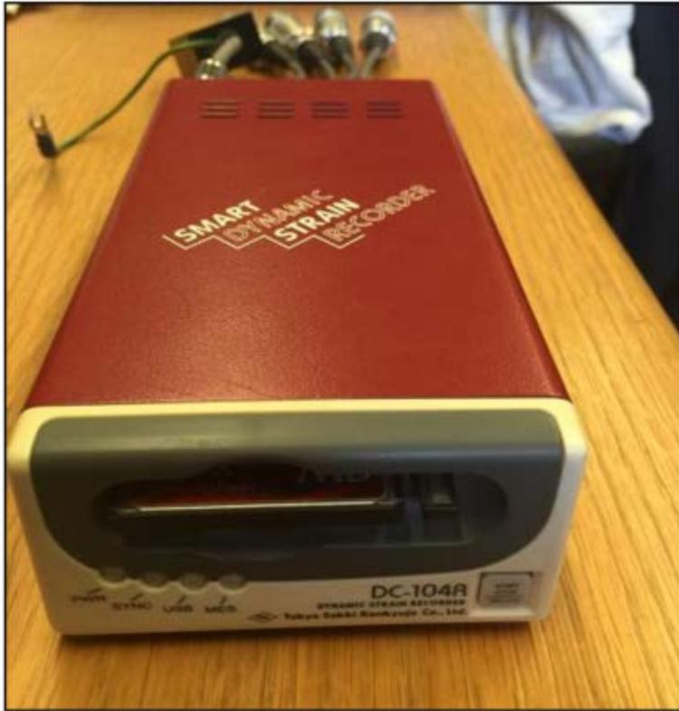
(a) Portable Dynamic Strain Recorder
