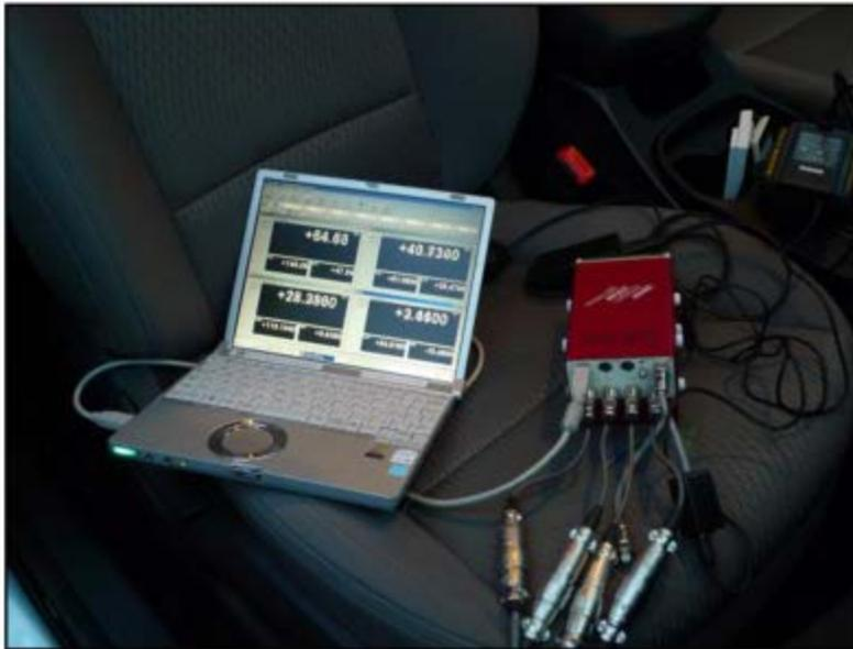
(b) Computer Controlled Data Acquisition System
