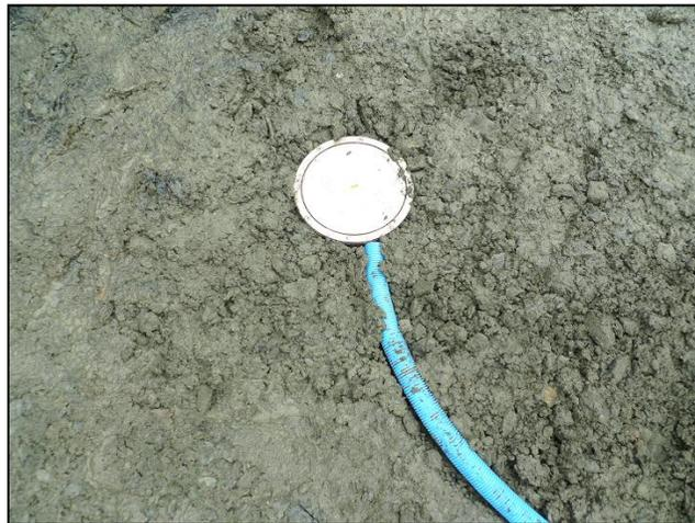
**Figure 30: Load Cell with Protected Cable**
