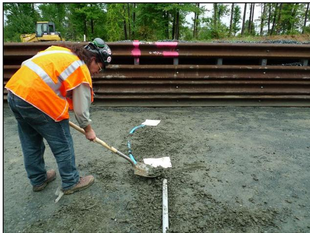
**Figure 32: Load Cells at Locations Under the Track, Covered by Sand Bags**
