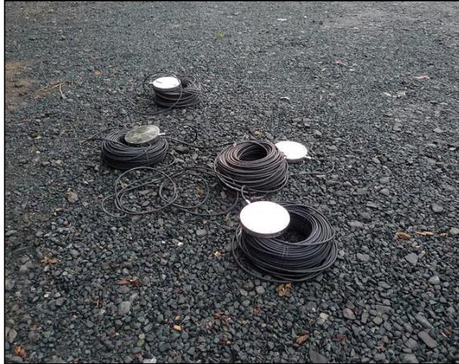
**Figure 29: Load Cells Ready for Deployment**
