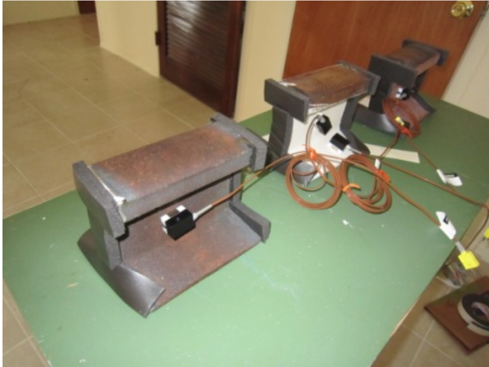
Figure 4. Uncoated and Coated Short Rail Segments
