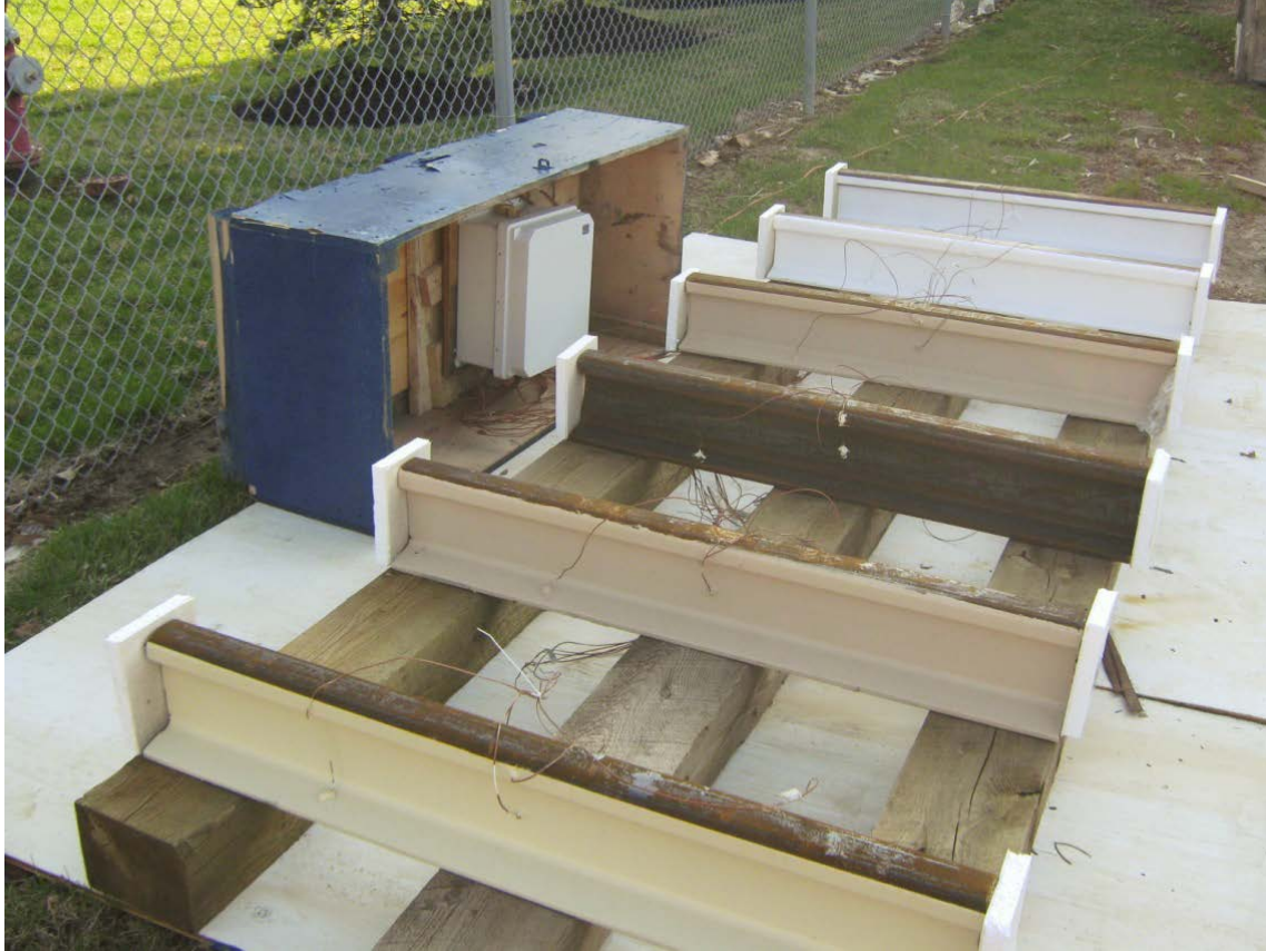
Figure 3. Coated Rails Exposed to Sunlight [20]
