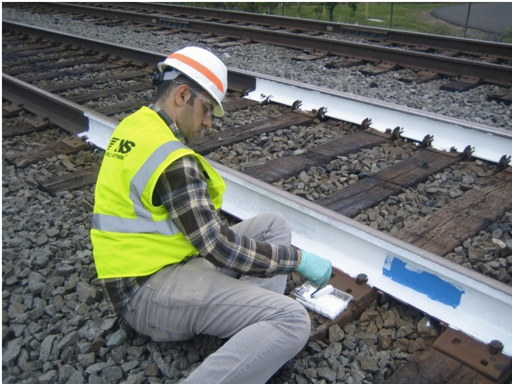
Figure 19. Applying White Coating on Red Metallic Primer (the Patch Area for Installation of the Sensor is Covered with Blue Painter's Tape)
