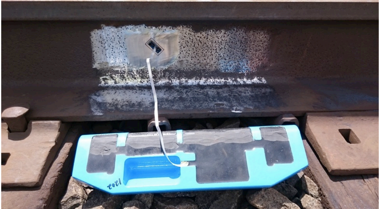
Figure 22. Sensor Installation on Rail with Coting Without Coating
