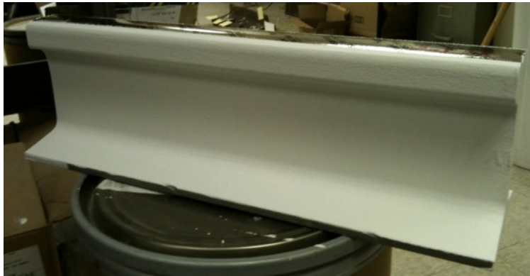
Figure 7. Coating on a 3-Foot Rail Segment
