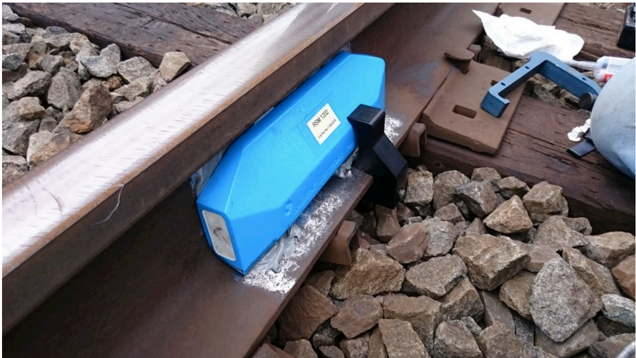
Figure 23. Completed Sensor Installation on Rail Without Coating
