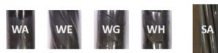
Figure 3. Representative prestressing wires (WA, WE, WG and WH) and strand (SA) in KSU tests.
