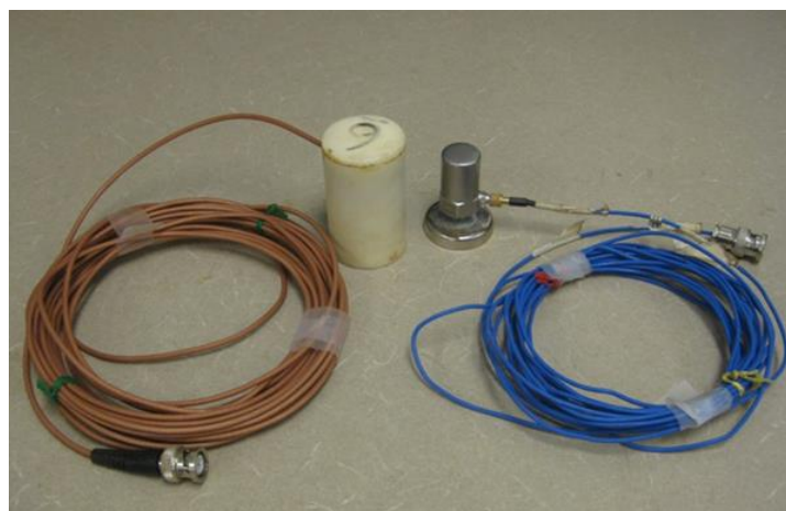
Figure A.2. Geophone and Accelerometer
