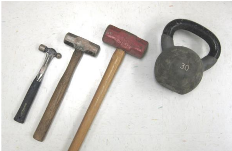
Figure 26. Impact Energy Sources (2-oz Ball-Peen Hammer, 3 lb. Sledgehammer, 10 lb. Sledgehammer and 30 lb. Kettlebell Weight)
