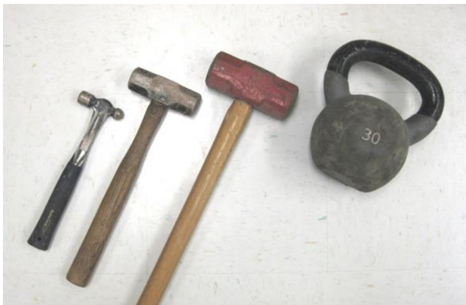
Figure A.4. Impact Energy Sources (2-oz Ball-Peen Hammer, 3 lb. Sledgehammer, 10 lb. Sledgehammer and 30 lb. Kettlebell Weight)
