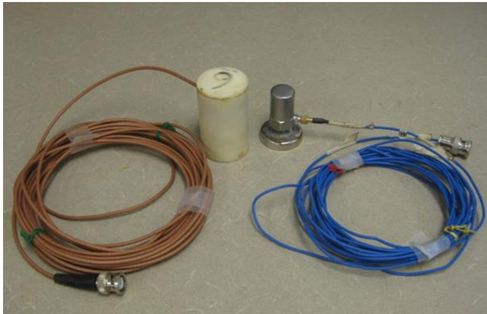
Figure 24. Geophone and Accelerometer
