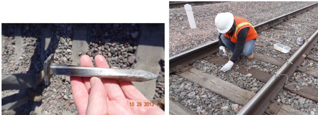
Figure 21. Metal Spike and Installation of Metal Spike for Coupling Accelerometers to Ballast
