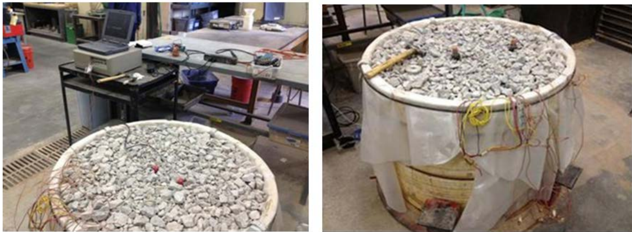
Figure 27. Setup of Small Scale Laboratory Ballast Testing Setup at UTEP
