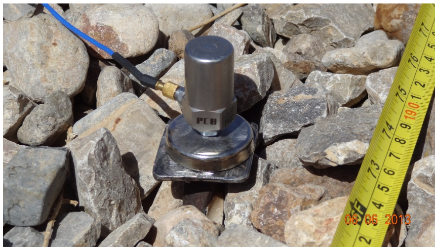
Figure 22. Accelerometer Attached to Top of Metal Spike Using a High Strength Magnet
