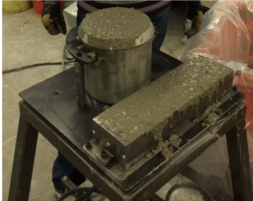
Figure 2.1. ASTM C 231-Compliant Container and one ASTM C 666-Compliant Freeze-Thaw Specimen Mounted to Custom Vibrating Table
