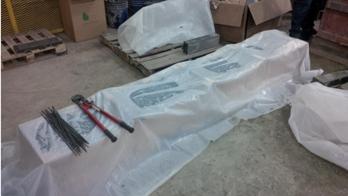
**Figure 10.26. Unreinforced tie covered in plastic**
