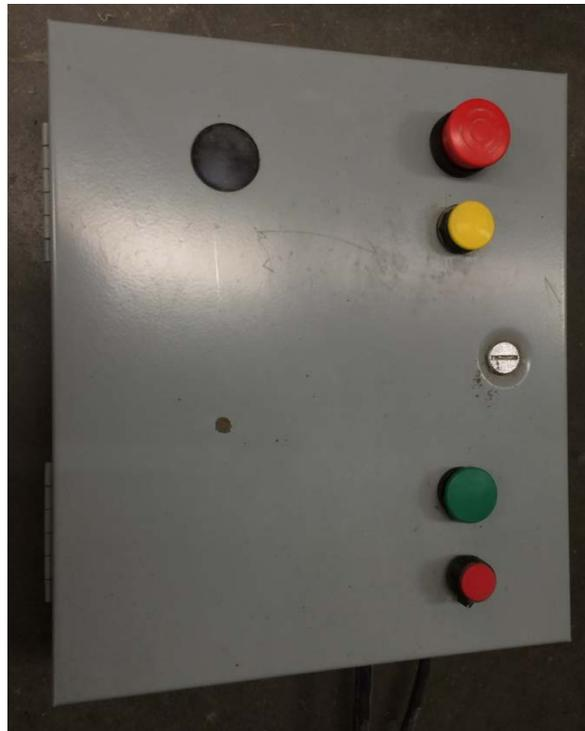
**Figure 5.18. Control unit for the large vibrating table**
