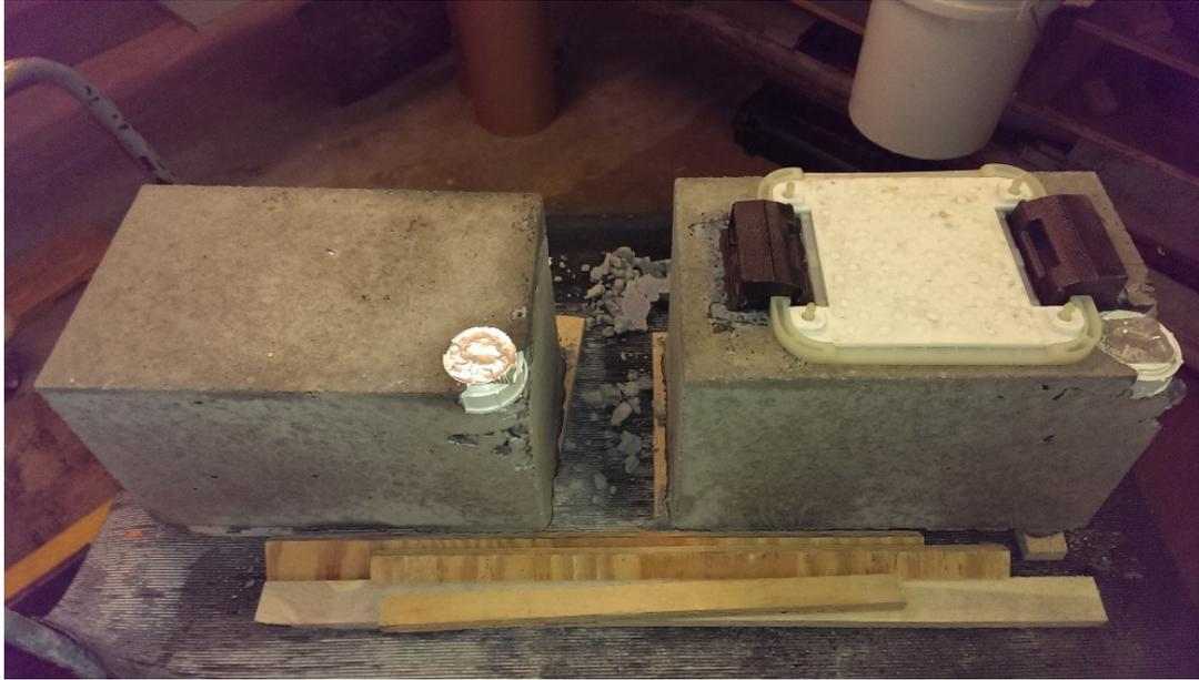
**Figure 8.12. De-molded model concrete cross-ties with PVC access plug where multi-conductor shielded cables are encased**
