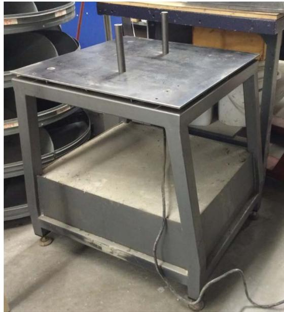
**Figure 5.16. Large vibrating table**
