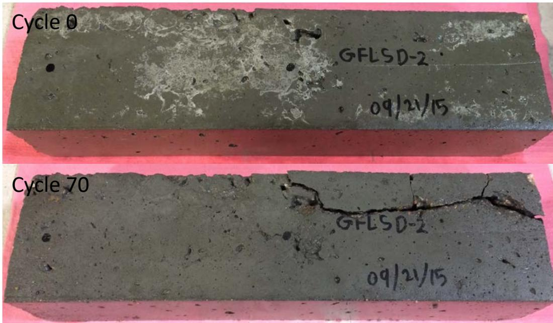
Figure 10.19 Cracked saw-cut sample (angle 1)
