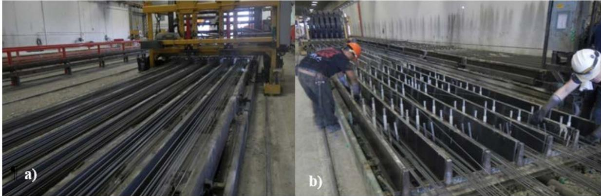
**Figure 6.4. a) Reinforcing steel wires during installation, and b) enforcing the wire spacing pattern in Plant A**
