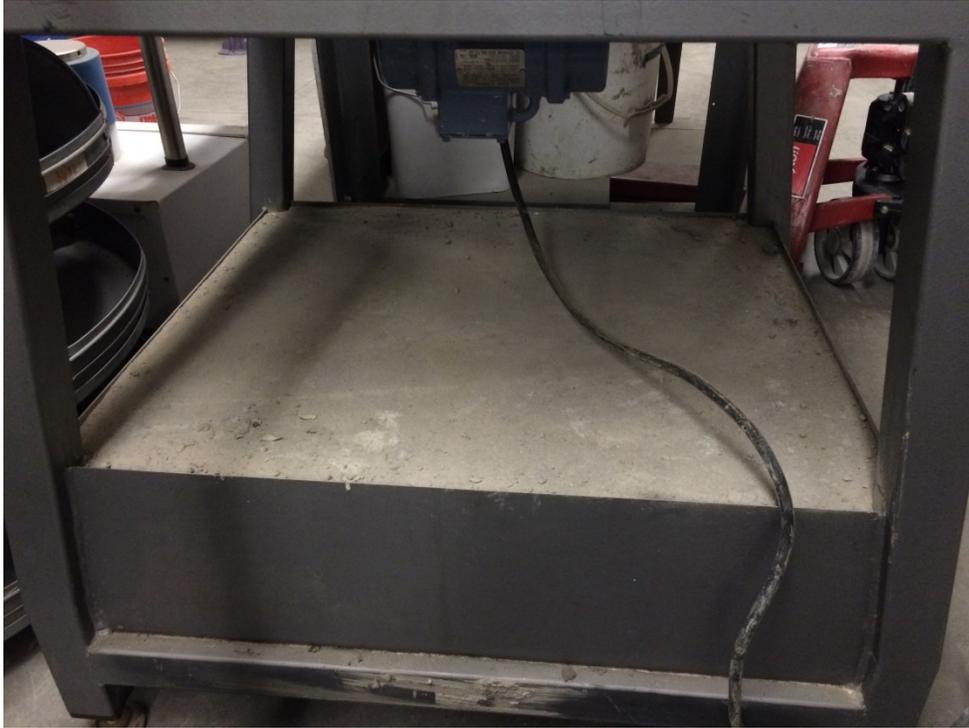
**Figure 5.21. Concrete block at the bottom of the large vibrating table**
