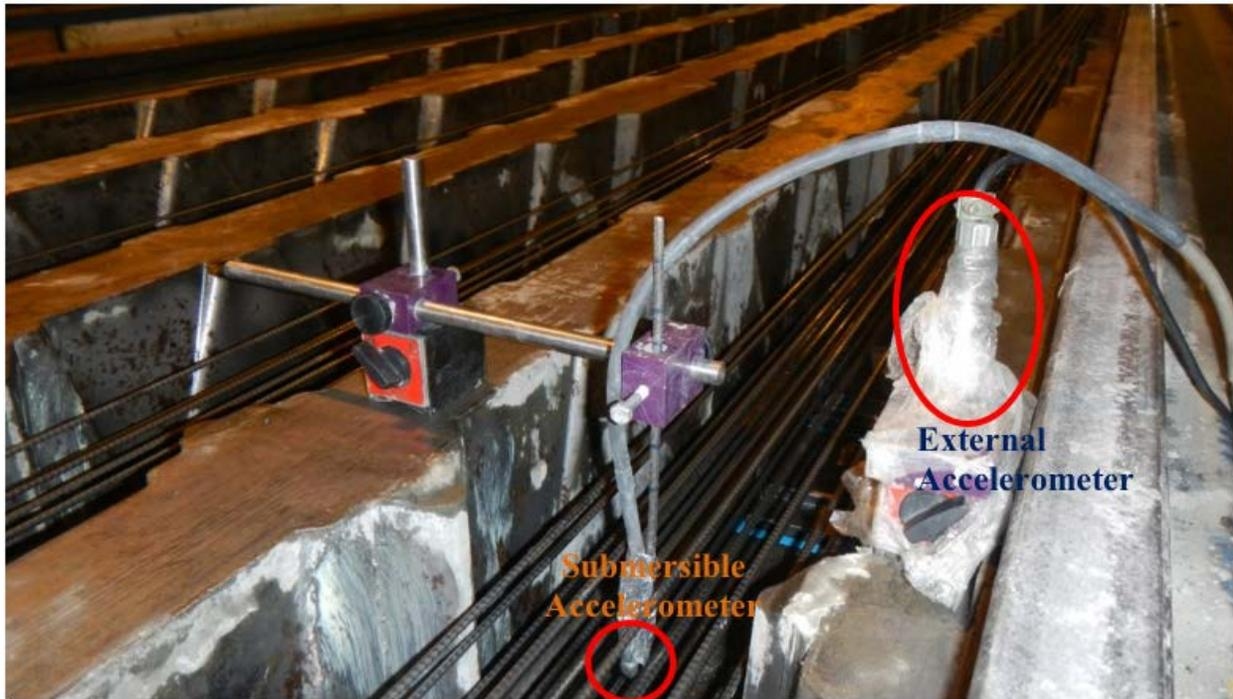
**Figure 6.10. Two accelerometers in position for recording**
