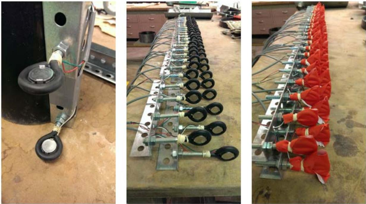
**Figure 7.3. Construction of iButton sensors (left), fitted with rubber bands (center), and covered in gore-tex fabric (right)**
