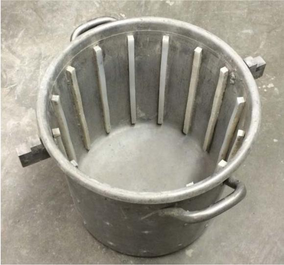
Figure 5.14. Rheometer concrete container
