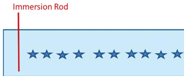
**Figure 4.4. Illustration of immersion pencil (probe) vibrator in 15.24 x 15.24 x 122 cm Plexiglas mold where stars represent the nominal location of an immersed accelerometer during vibratory testing**
