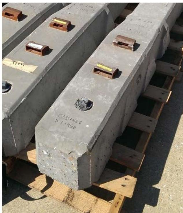
**Figure 7.5. De-molded concrete cross-ties with square cap added to PVC access plug where multi-conductor shielded cables are encased**
