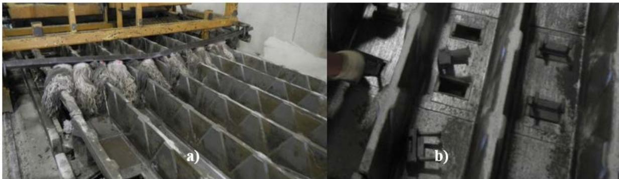
**Figure 6.1. a) Forms cleaning and oiling, and b) shoulder installation in Plant A**
