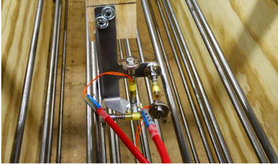
**Figure 10.24. Vibration wire gauges inside the ties**
