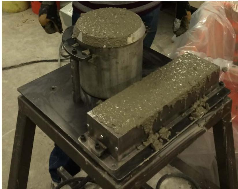
**Figure 5.25. The small vibrating table**
