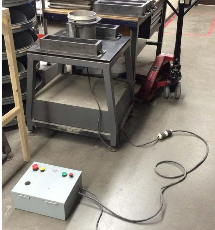
**Figure 5.24. The large vibrating table with two freeze-thaw specimen molds and ASTM C231 specimen container bolted to the table top**
