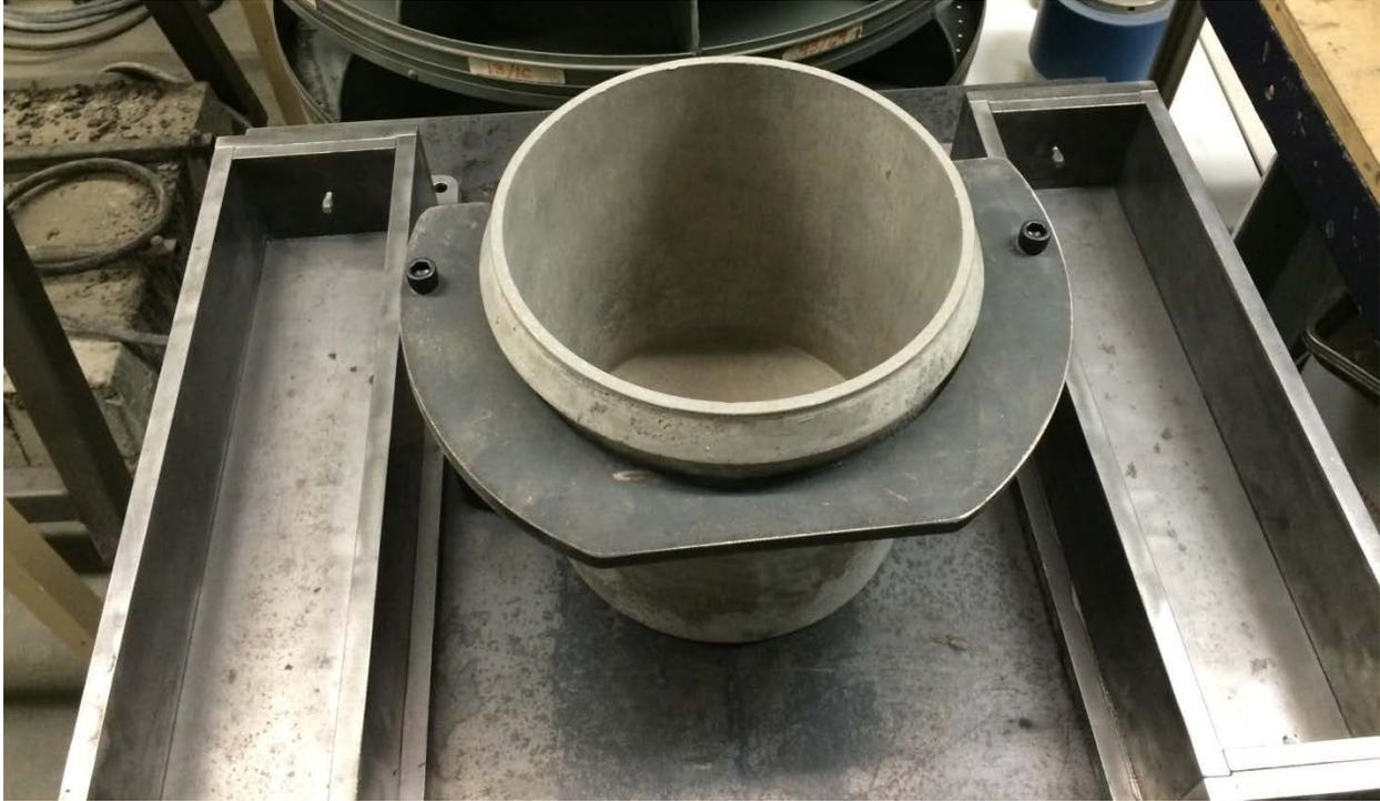
**Figure 5.23. ASTM C231 concrete air content container bolted to the top of the large vibrating table**
