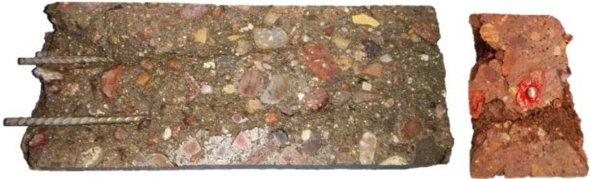
**Figure 10.10.** Mass loss for saw-cut samples in freeze-thaw testing (SHT4)
