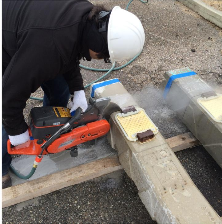
**Figure 10.4. Saw-cutting samples from the tie end**
