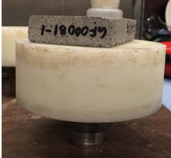
**Figure 5.30. A concrete sample fixed to the plastic cylinder**
