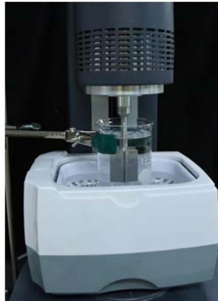
**Figure 3.4.** Shaker table for concrete vibration (left) and ultrasonic bath for the vibration of the surrogate yield-stress fluid, granular material, and mortar (right)
