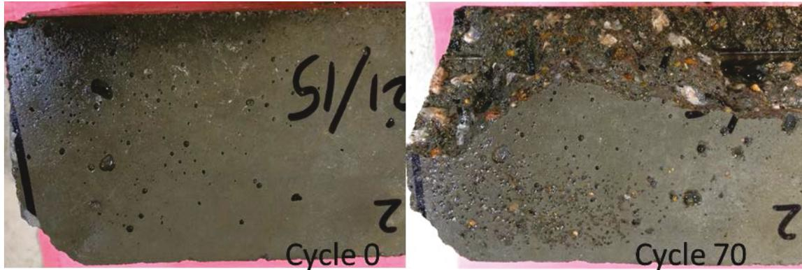
**Figure 10.23. Cracked saw-cut sample (angle 5)**
