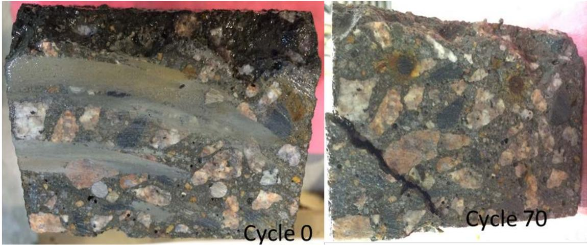
**Figure 10.21. Cracked saw-cut sample (angle 3)**
