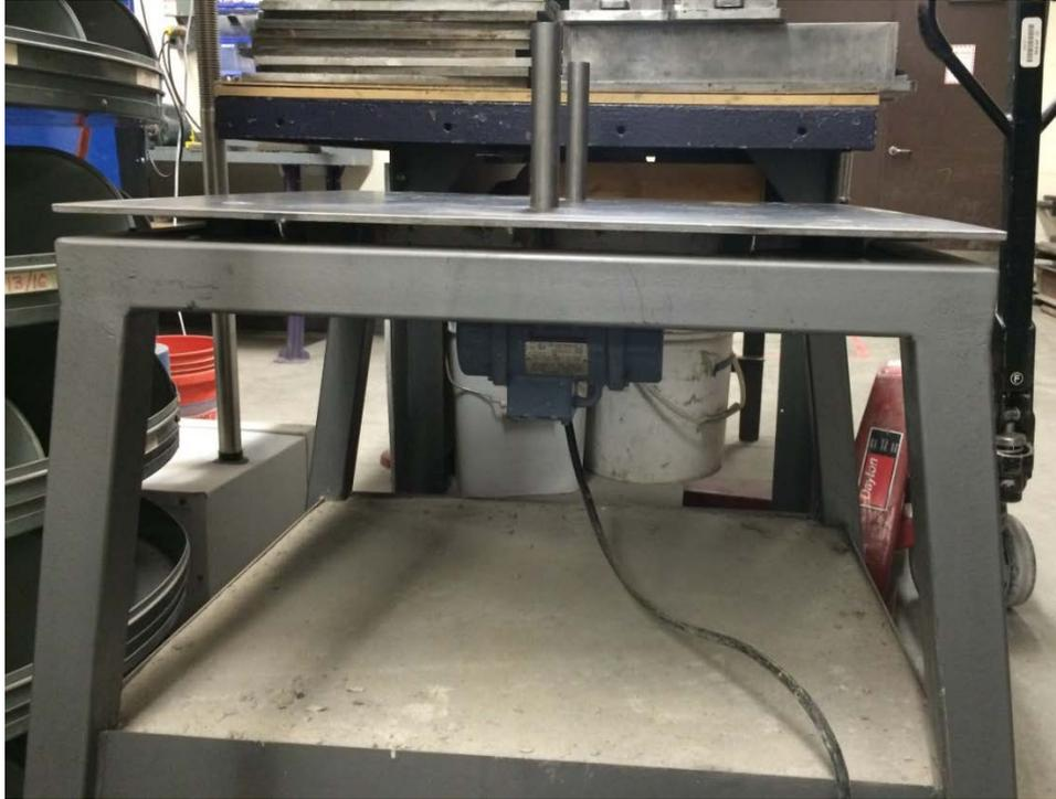
**Figure 5.19. Vibrating motor attached to the bottom of the table top**
