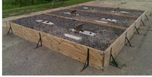
**Figure 7.7. Construction of ballast box (left) and final configuration (right)**
