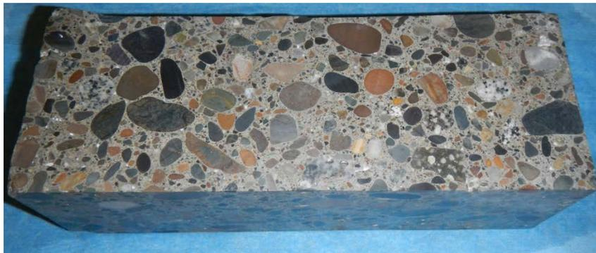
Figure 10.6. Typical 4 x 3 x 11 in. saw-cut freeze-thaw sample
