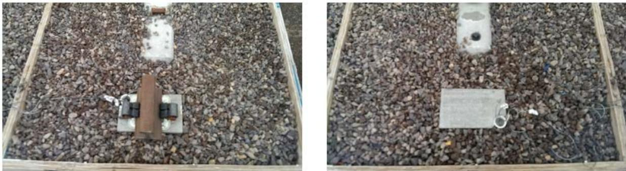
**Figure 8.13. Model cross-ties installed in model ballast in Rantoul, IL**
