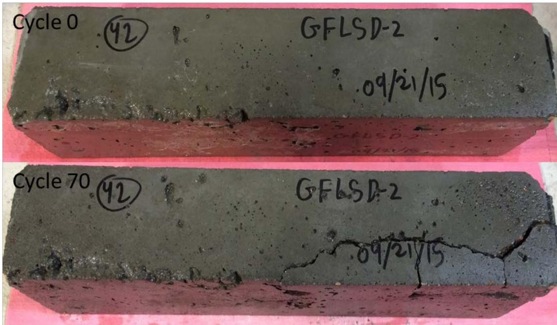
Figure 10.20. Cracked saw-cut sample (angle 2)
