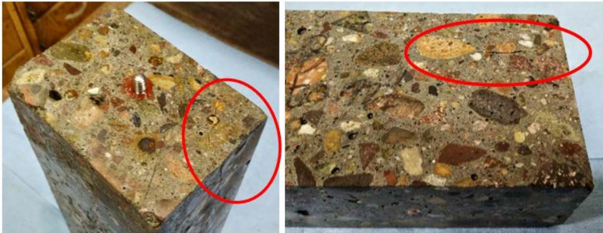
**Figure 10.8. Cracking pattern in saw-cut samples in freeze-thaw testing (SHT3)**
