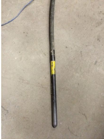
**Figure 5.17. Immersion vibrator**
