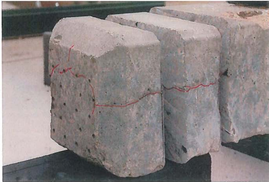
Figure 23. Opposite side view of two sections removed at 4 inches and 8 inches from south end of tie NDT #7. L3672 102312 20
