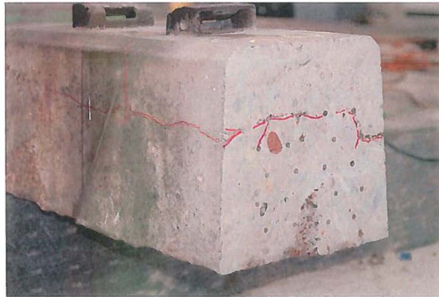
Figure 44. Oblique side view of tie NDT #2 after removal of 10 inches at end.
