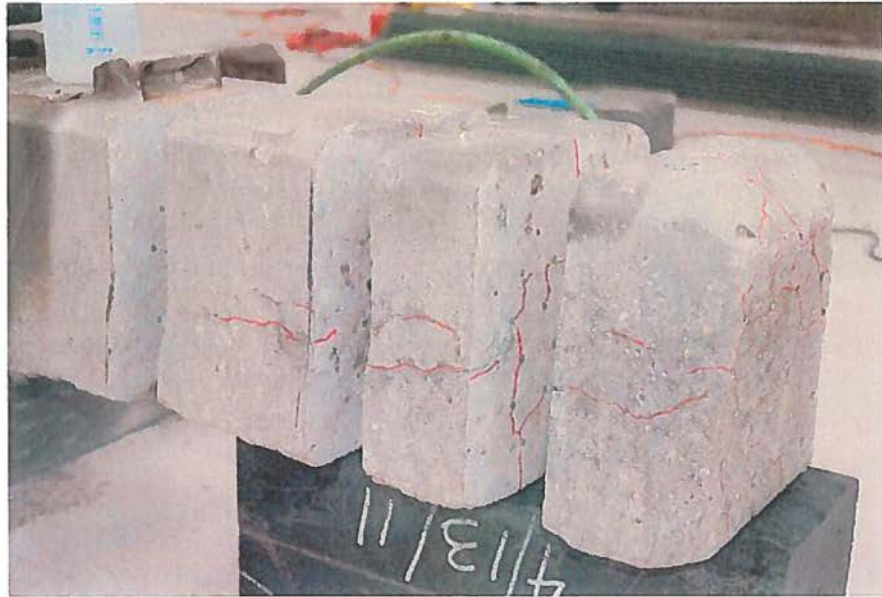
Figure 33. Opposite side oblique view of successive sections removed at north end of tie NDT #69. L3672 102312 43
