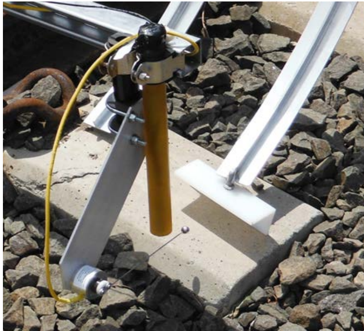
Figure 18. Ball End “Tapper” Installed on ACTT-2
