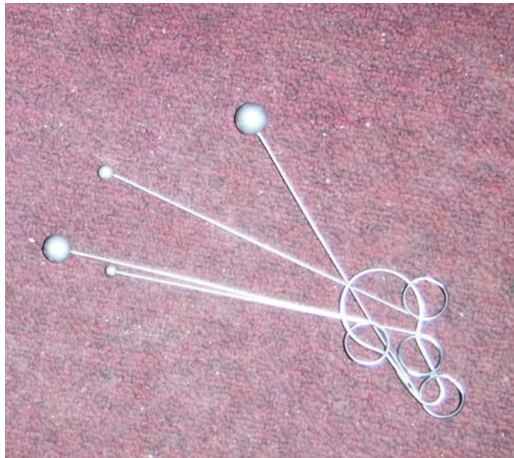
Figure 17. Ball End Impactors
