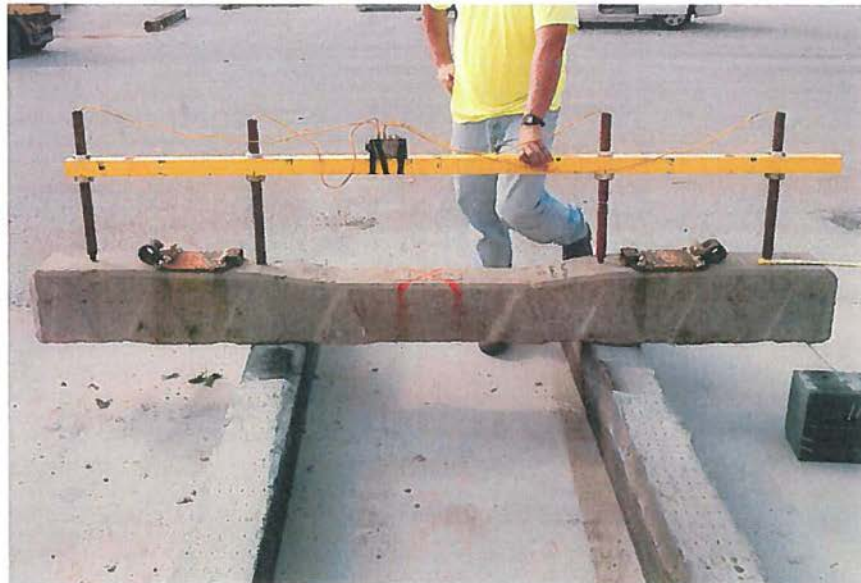
Figure 26. Tie NDT #69 with transducer array placed as employed in making impact echo recordings, rated by NDT as condition "2" both ends. L.3672 102312 30
