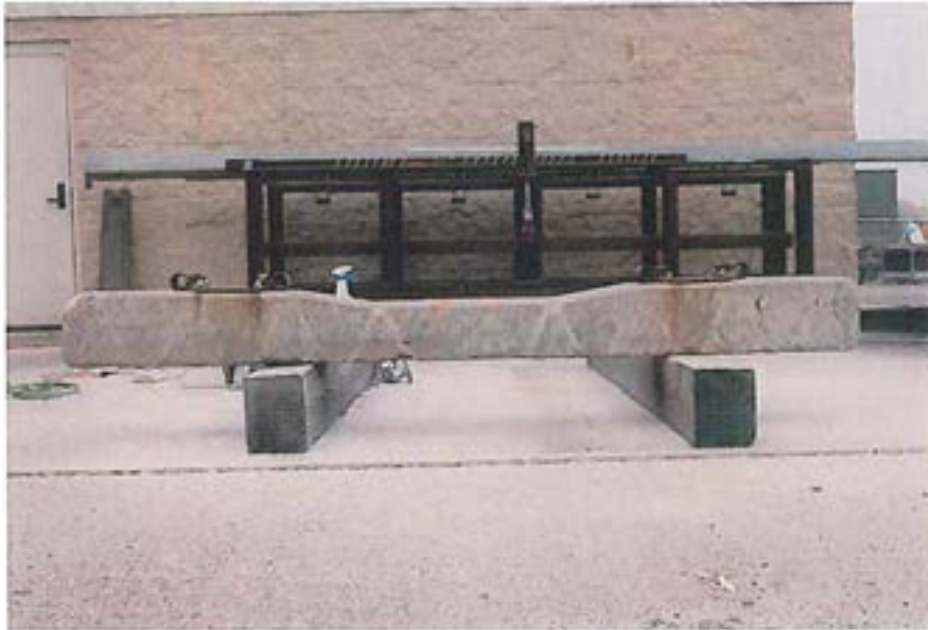
Figure 55. Overall view of tie NDT #1 rated by NDT as condition "2" on north end, and condition "3" on south end. L3672 102512 71
