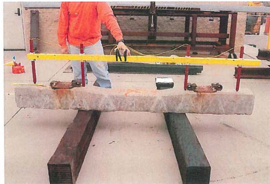
Figure 2. Tie NDT #7 with the NDT transducer array positioned on the top of the tie as employed in the impact echo testing. L3672 102312 16
