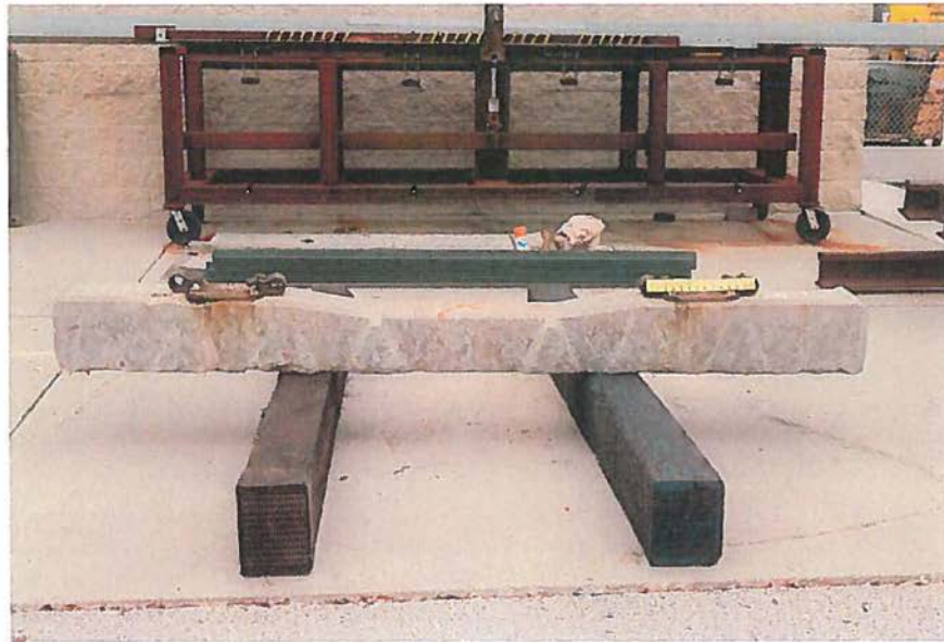
Figure 1. Side view of prestressed concrete railroad tie identified as NDT #7, manufactured by CXT at Grand Isle, Nebraska in 2006. L3672 102312 01
