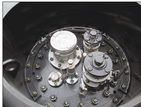
Typical arrangement found in the protective housing on the CPC-1232 and DOT-117 cars.
