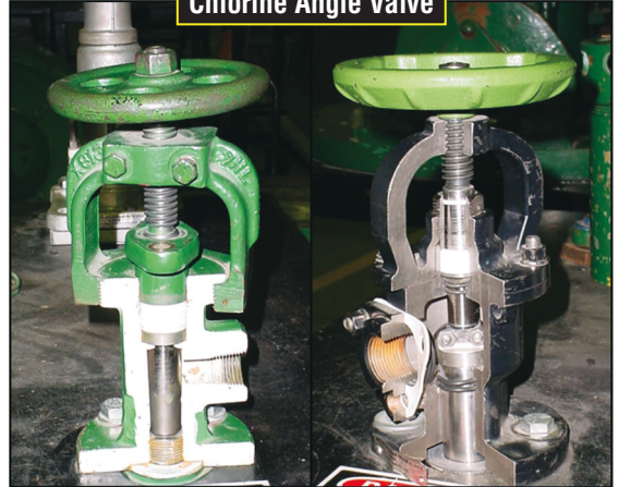
Chlorine Angle Valve
