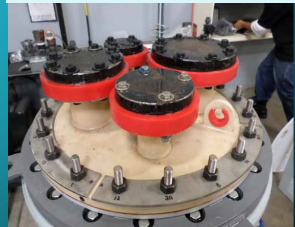
UHMW PE Flange Faces & PVDF Coating
