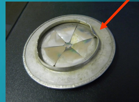
Dented Rupture Disc Lip
