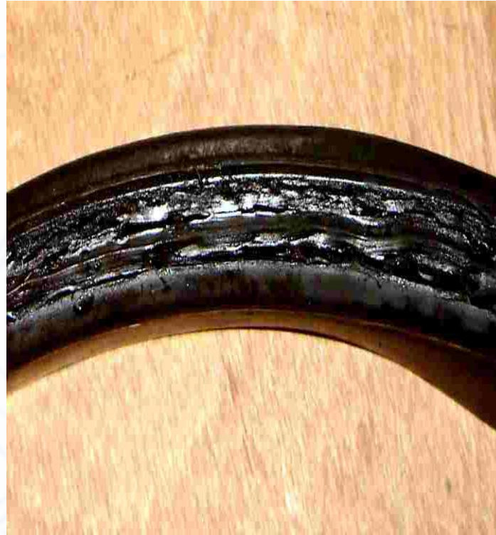
Viton® in Asphalt [Viton® 450°F, Asphalt = 400°F]
