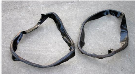
Buna-N (Nitrile) in Asphalt [Buna-N = 200°F, Asphalt = 400°F]
