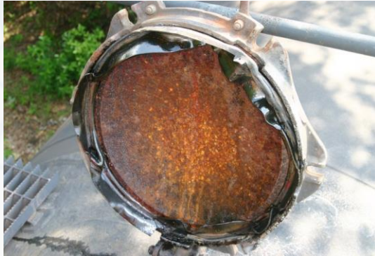
Buna-N (Nitrile) in Asphalt [Buna-N = 200°F, Asphalt = 400°F]
