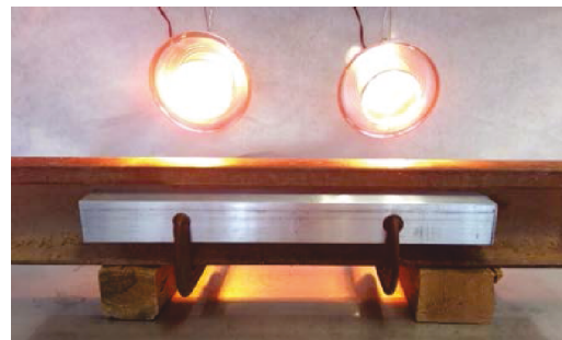
Figure 3. Testing setup using radiative heating to thermally cycle one yard rail sections with RTCS prototype device.
