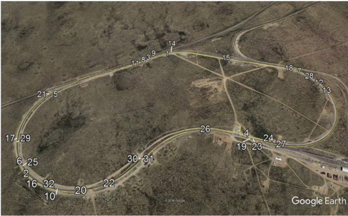
Figure 5. HTL with Broken Rail Locations
