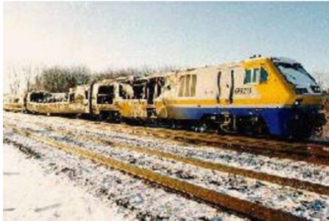
Figure 2-4. Photograph from Incident in Brighton, ON, Showing Fire Damage to Rail Cars
