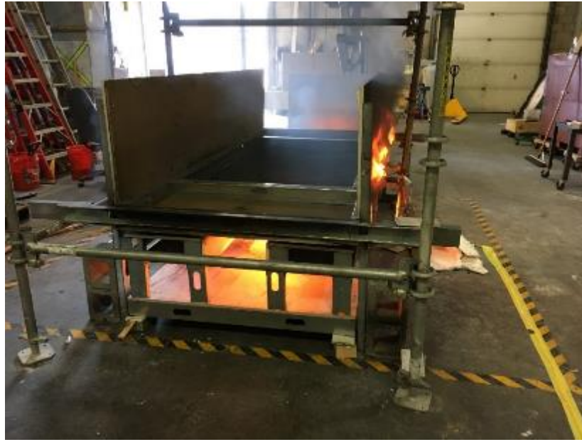
Figure 3-11: Steel Test Series, Diesel Fire, Channel Configuration.
