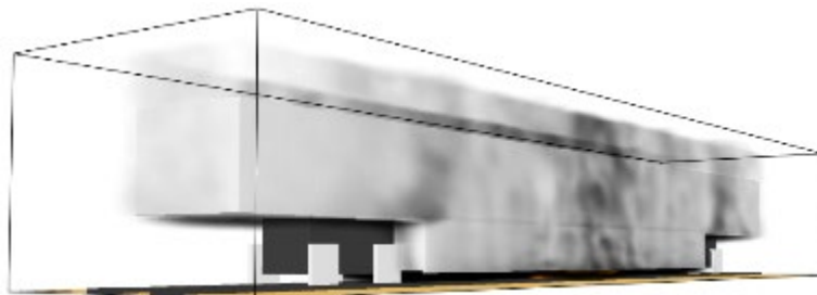
Figure 6-39. Visualization of HRRPUV and Soot Production for Model 6 (Gasoline Spill Fire) Simulation
