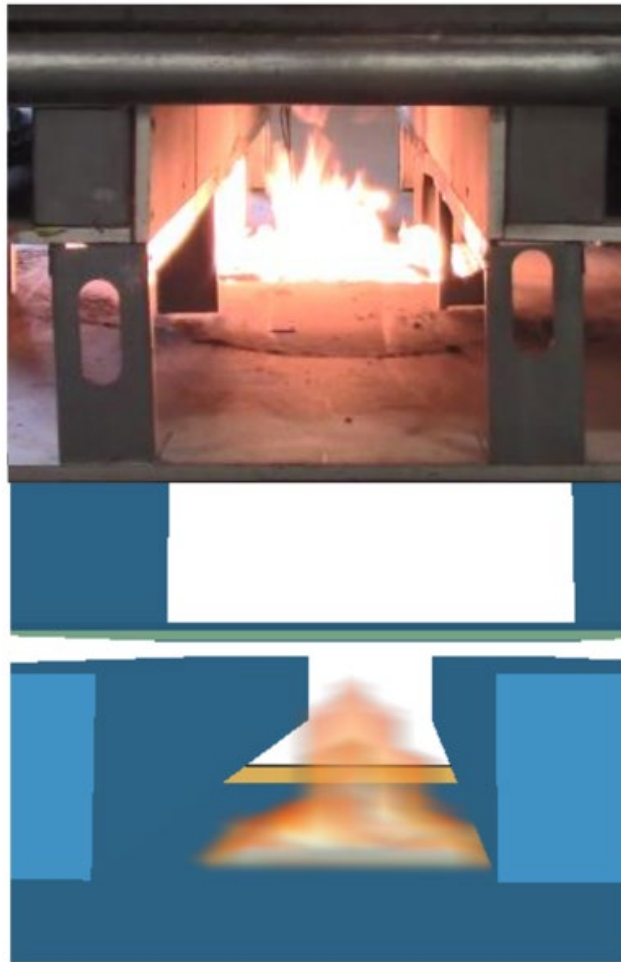
Figure 4-17. Fire Flame of Testing (Top) and FDS Simulation (Bottom) at the Time of 10 Minutes for Obstructed Configuration/Trash Fire
