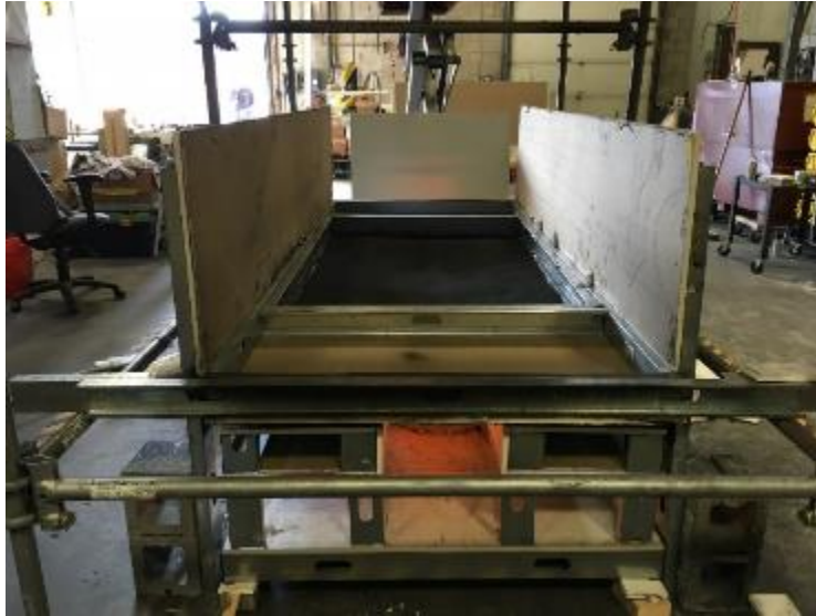
Figure 3-10: Steel Test Series, Trash Fire, Channel Configuration.
