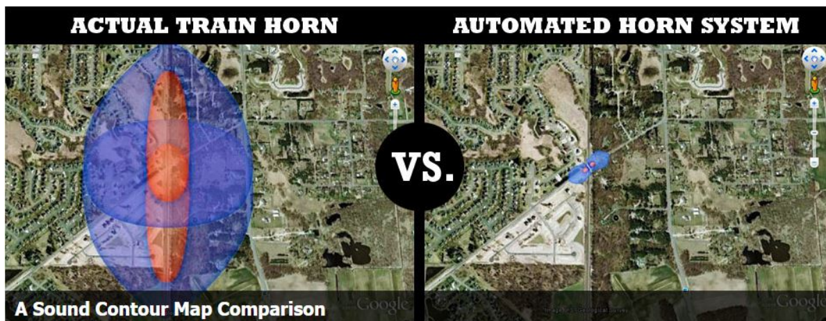
Figure 7. Sound Contour Map Comparing a Train Horn Sound with an AHS
