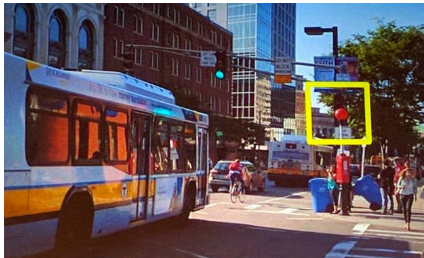
Figure 17. Red Balloon on a White Stick Identified by Google Self-Driving Car Interpreted as a Red Light
