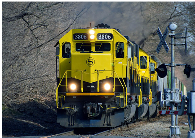
Figure 5. Locomotive with Headlights Forming a Triangle, as Required by the FRA
