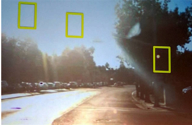
Figure 19. Google Self-Driving Car Detecting Multiple Lights on a Sunny Day Scenario
