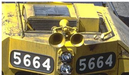
Figure 6. Air Horns Installed on the Roof of a Diesel-Electric Locomotive
