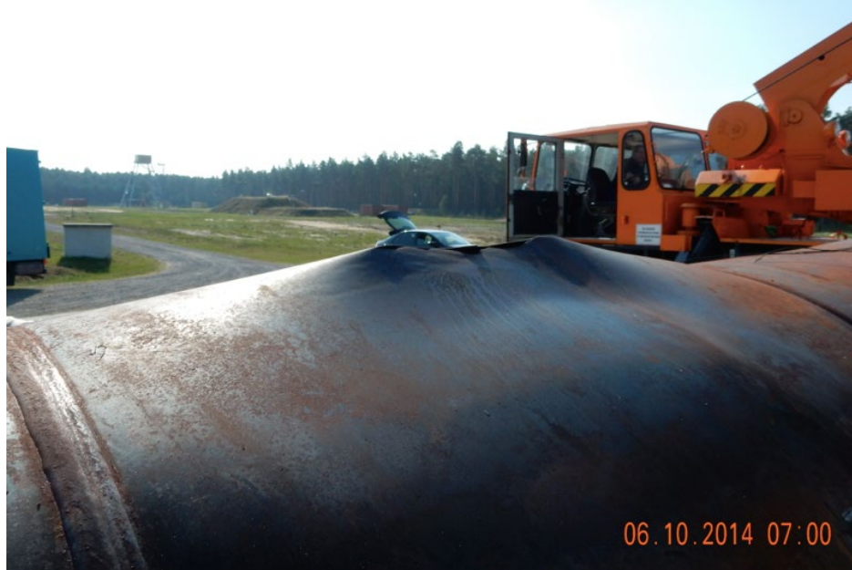
Figure 54. Test 1b - View of Vessel Rupture.
