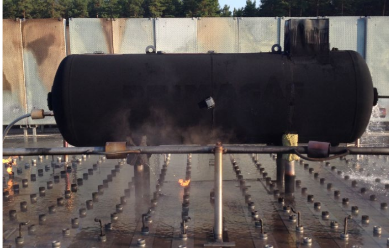
Figure 10. Picture of the Fire Calibration Test Tank and Setup
