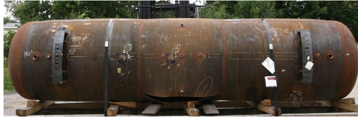
Figure 3. Burst Hydrostatic Tested Tank – Overview
