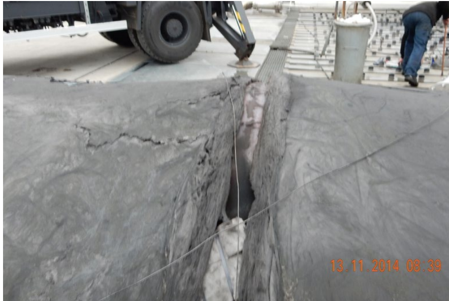
Figure 90. Test 5 with View of Open Gap in Insulation Note significant local plastic deformation to tank wall.
