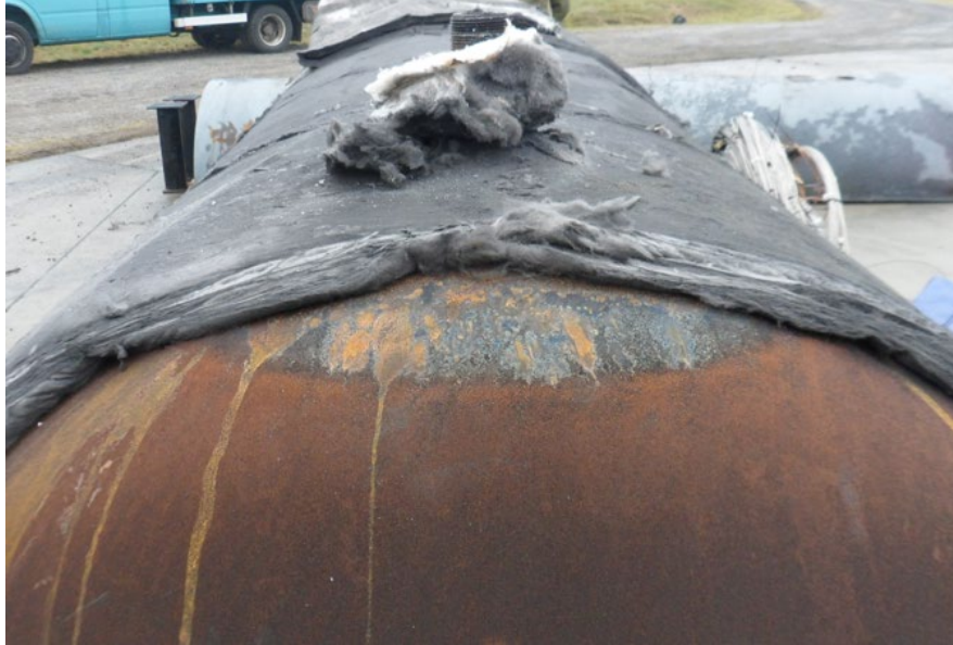
Figure 70. Test 3 - End View of Tank after Test. Note Liquid Level Mark on Tank. Note insulation on end dropped down.
