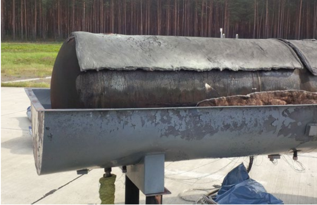
Figure 43. Test 1 - View of Dropped Down Insulation on West End and South Side
