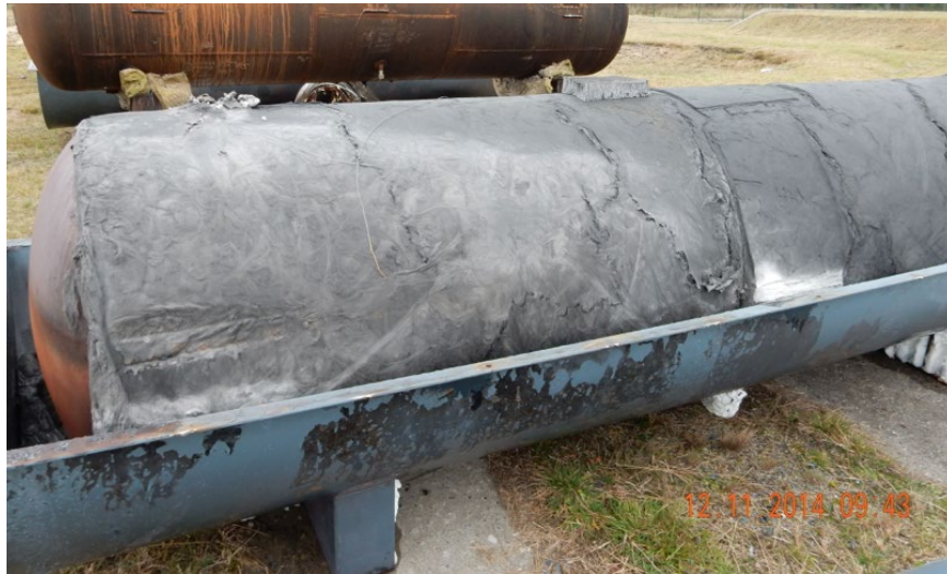
Figure 24. Test 4 - Note Double Layer of Insulation at Mid Span
