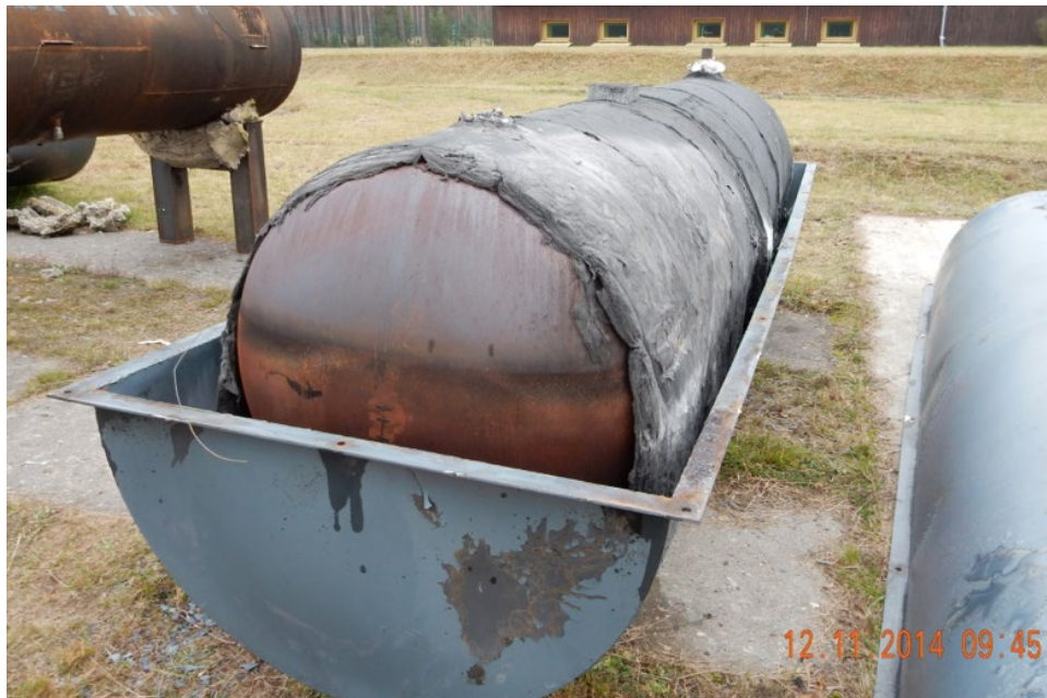
Figure 81. Test 4 - End view after Jacket Removal. Note liquid level markings on tank end. Tank was probably filled to 66%
