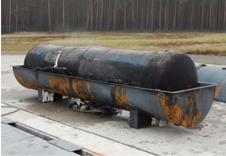
Figure 92. Test 5 Showing Tank with Plastic Deformation near Mid Span.
