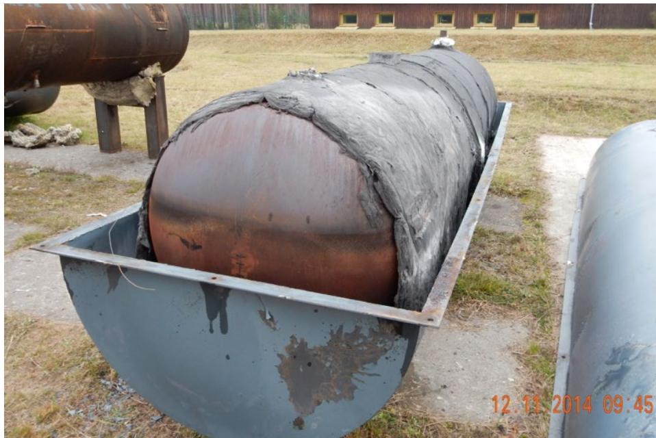
Figure 25. Test 4 - End View after Jacket Removal Note liquid level markings on tank end. Tank was probably filled to 66%
