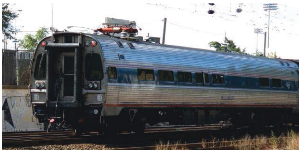
Figure 29: Amtrak's Manned Inspection Vehicle, Amtrak 10002
