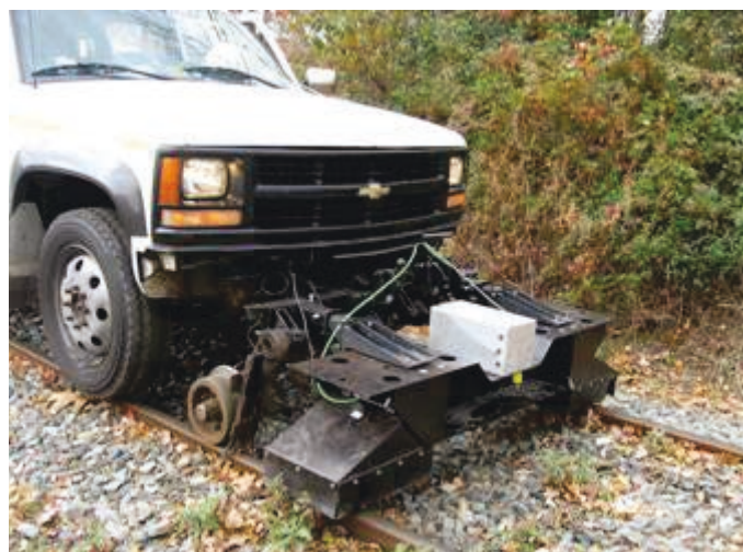
Figure 11: ATGMS Proof of Concept Testing on a High-Rail Vehicle
