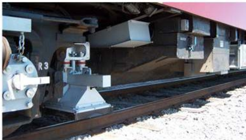
Figure 24: ATGMS Installation on DOTX 221
