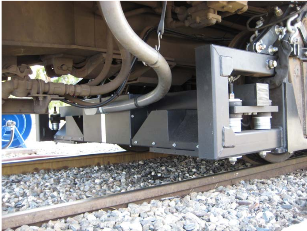
Figure 3. FRA ATGMS Installation on Amtrak Superliner II in Auto Train Service
