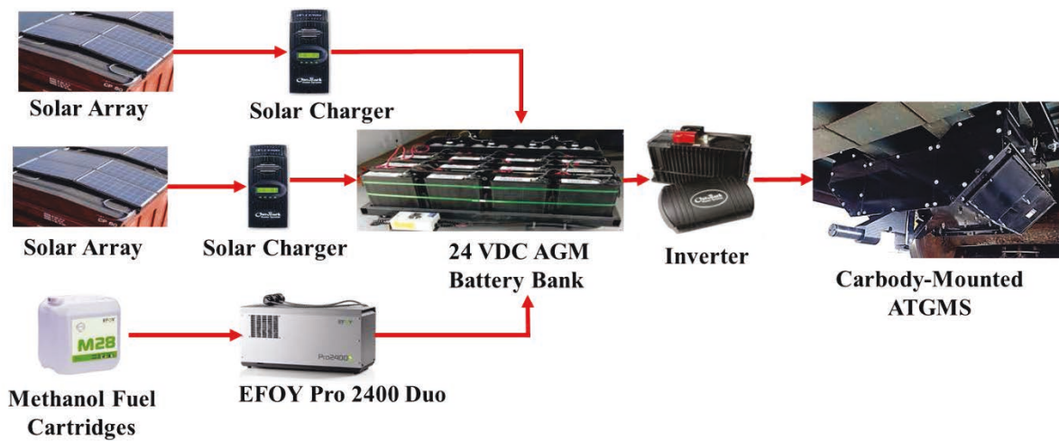
Figure 48: DOTX 225 ATGMS Power System Architecture
