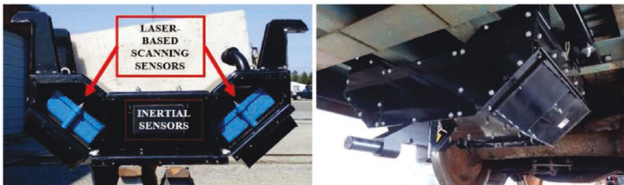
Figure 45: DOTX 225 Geometry Measurement Beam
