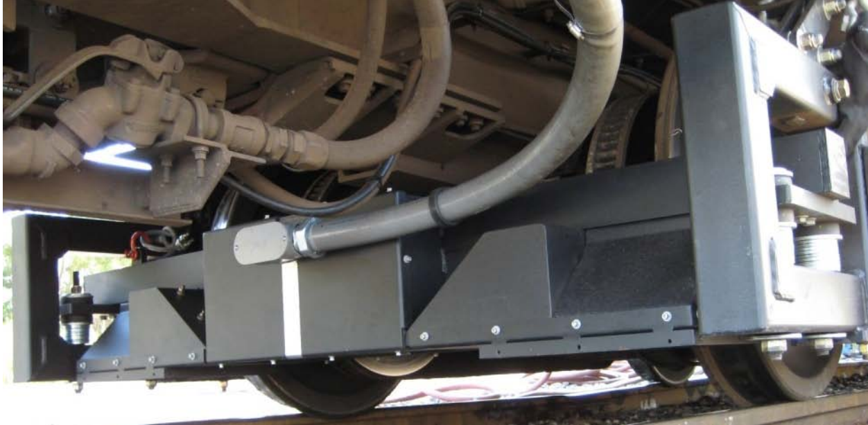
Figure 2. FRA's Truck-Mounted Pilot ATGMS on Amtrak Superliner 39000
