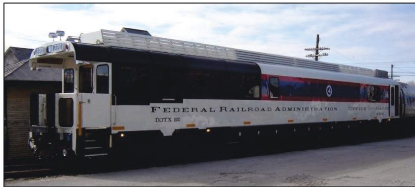
Figure 21: ATIP Manned Geometry Inspection Vehicle—DOTX 220
