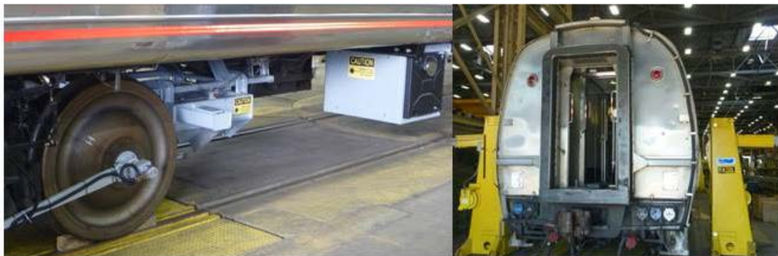
Figure 38: Stage 3 Carbody-Mounted ATGMS Installation, Amtrak's 82602
