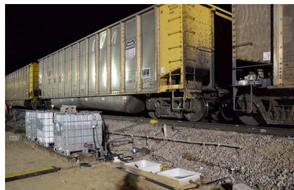
Figure 1. A water system at the Rainy Section at FAST as a train passes.
