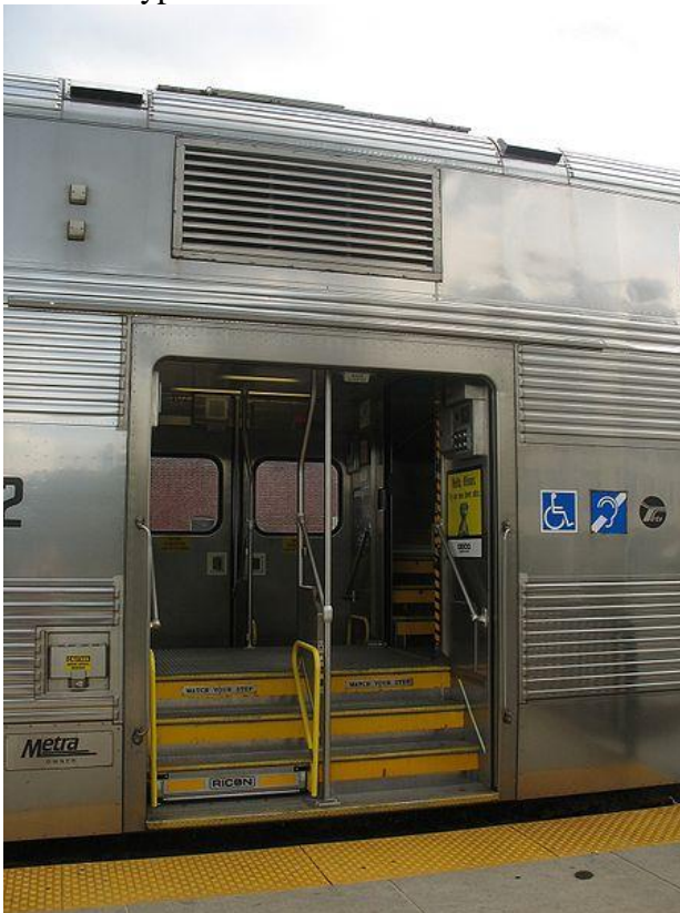
Photo 13. Metra Bi-Level Diesel District Center Entrance; Includes Car-Borne Wheelchair Lifts Manual Bypass Mechanism is Located to the Left of the Doorway.
