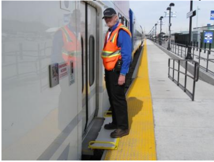
Photo 10. Bridge Plate Manually Deployed on Sound Transit
