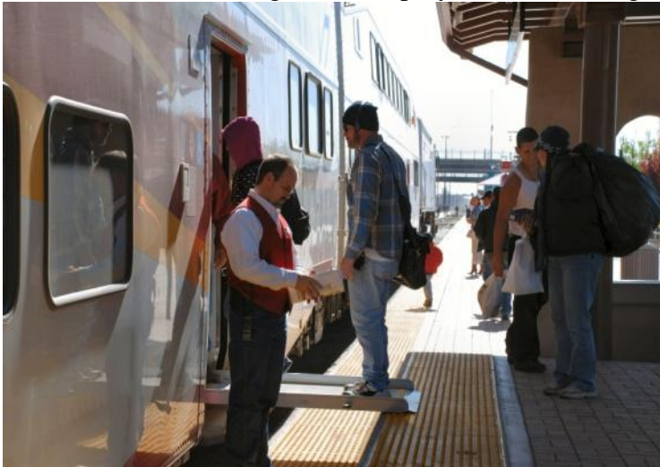
Photo 14. Manual Bridge Plate Deployed at a Mini-High
