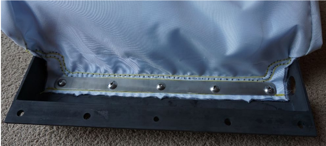
Figure 23. SIPS Airbag Attachment with Bolt Plate
