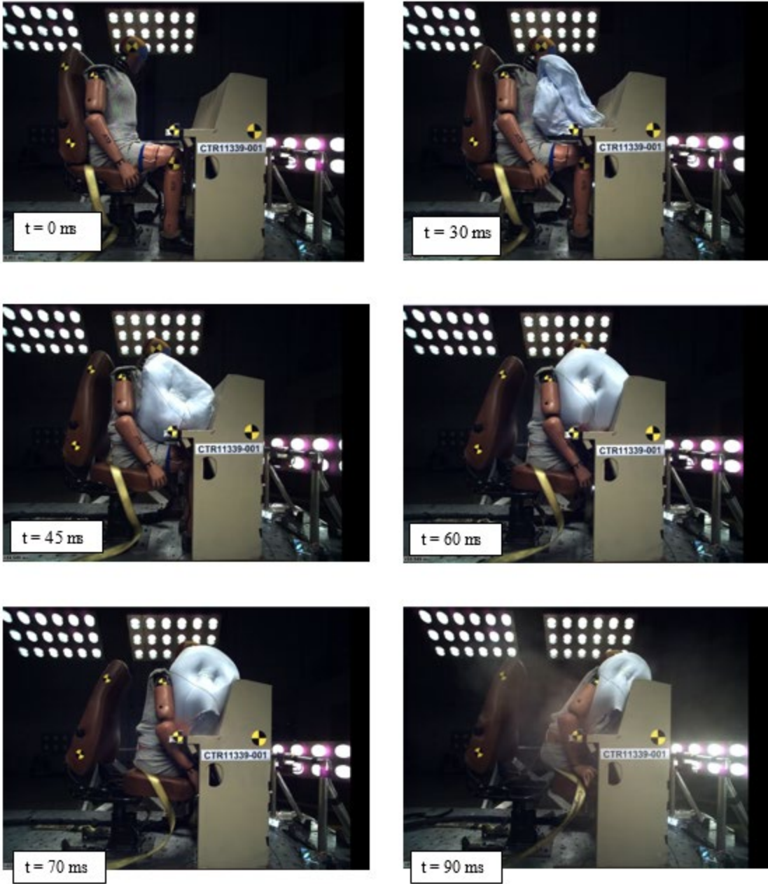
Figure 48. ATD Kinematics from Sled Test
