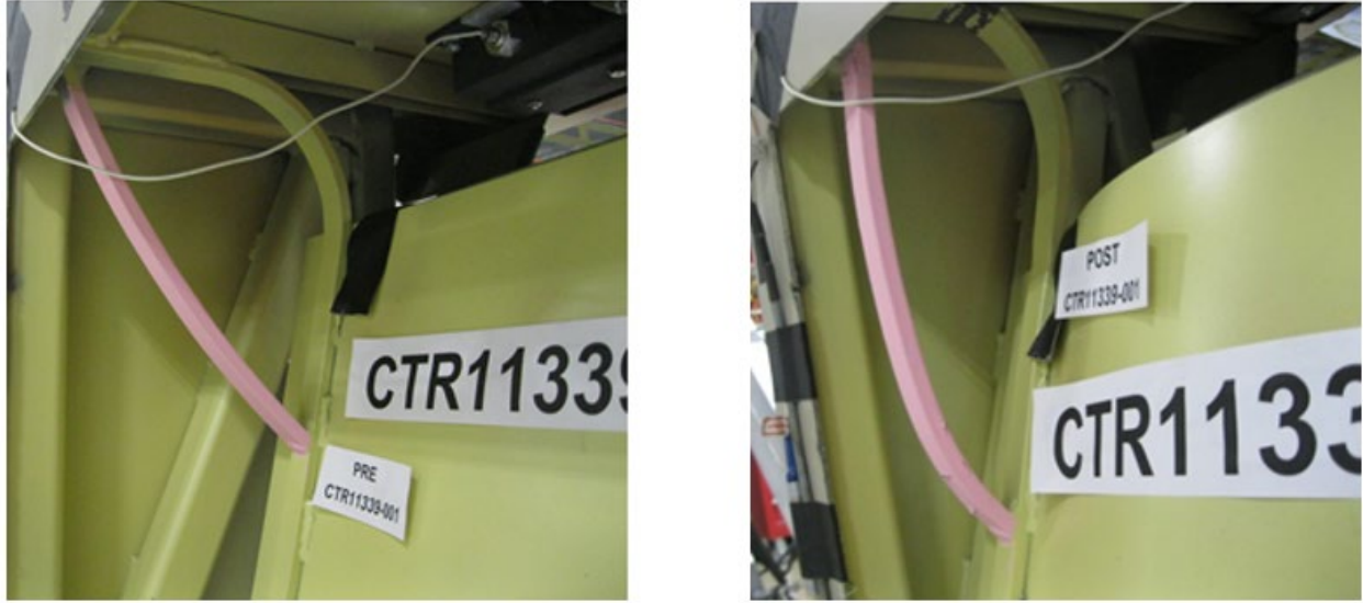
Figure 50. Permanent Deformation on the Knee Bolster Plate and Brackets (Left Pretest, Right Posttest)
