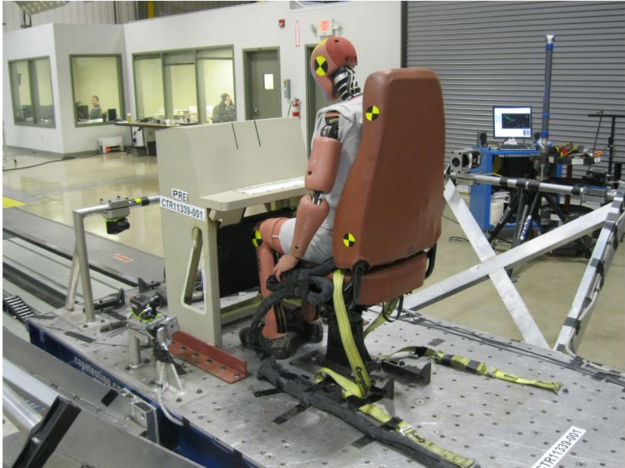
Figure 46. Overall Sled Setup with ATD, Prior to Crash Test
