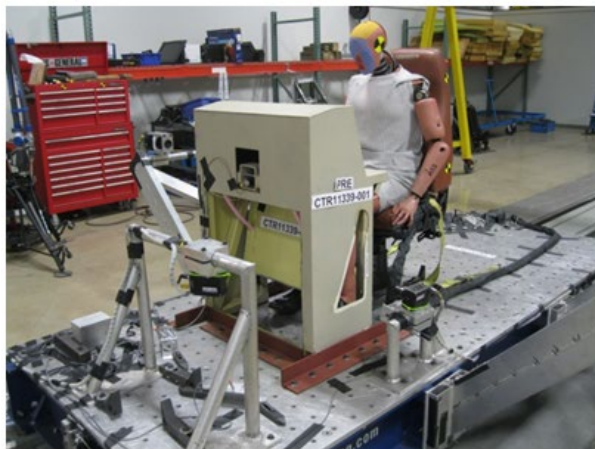
Figure 45. Sled Test Setup—Right and Left Views
