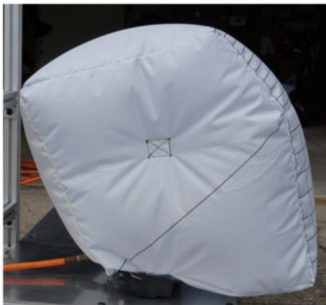
Figure 16. Compressed Air Inflation of the Airbag to Ascertain Geometry and Shape
