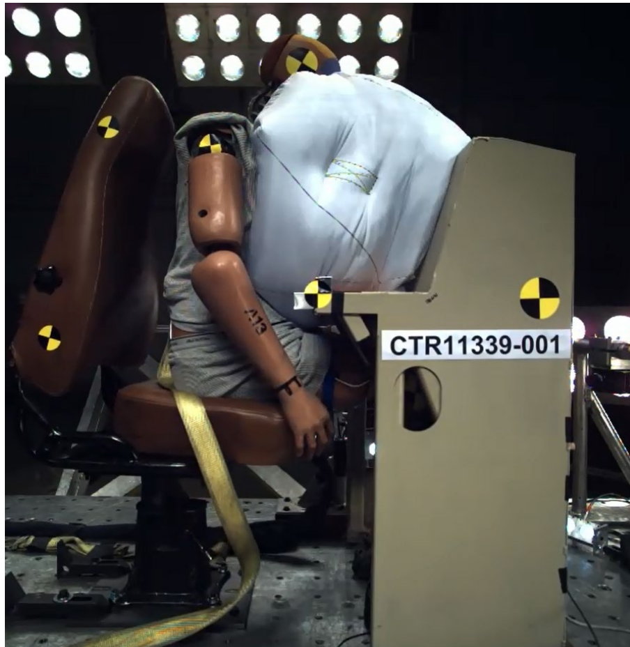
Figure 22. Airbag Geometry During Sled Test
