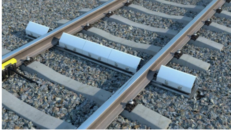
Figure 3-9. An example of a Dragging Equipment Detector (DED) [3]
