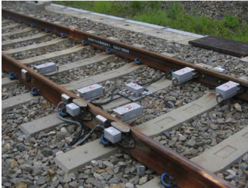
Figure 3-8. Another type of wheel crack detector deployed in Europe using Electromagnetic Acoustic Transducers [9]
