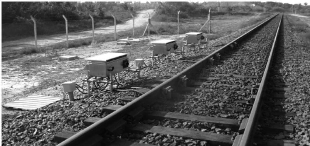
Figure 3-14. Triple-box configuration of a TBOGI-HD system [47]
