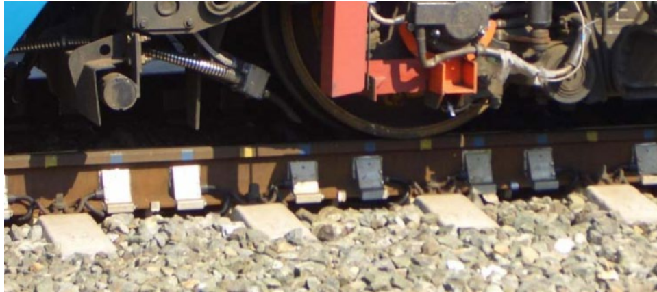
Figure 3-20. WIM strain gages attached to the web of the rail on an instrumented track [9]
