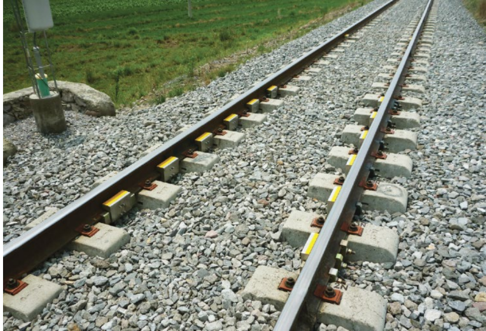
Figure 3-21. Strain gages of WILD system attached to the inner sides of rail web [65]
