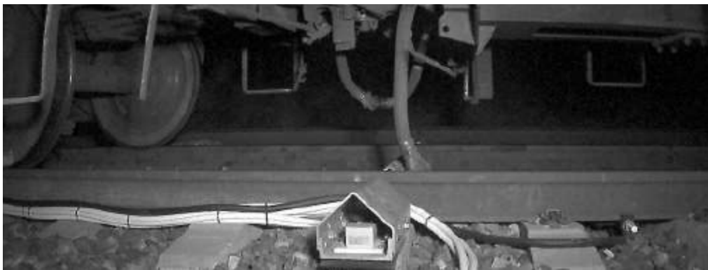
Figure 3-10. A dragging component detected by DED system [10]
