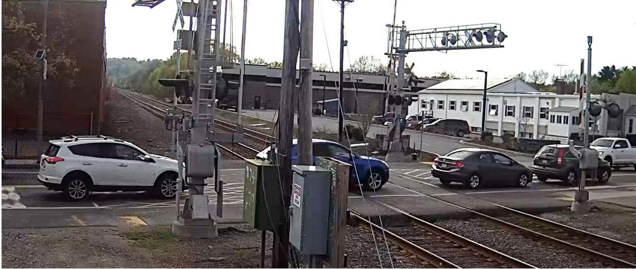
**Figure 10. Northbound Vehicles Stopping on Tracks Due to Congestion**
