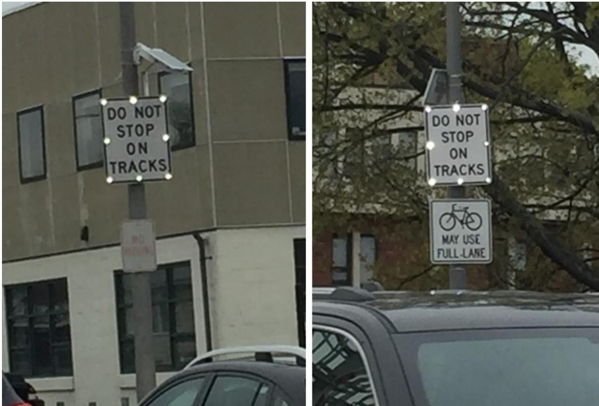
**Figure 8. TAPCO (left) and TSC (right) Signs from Approximately 90 Feet**
