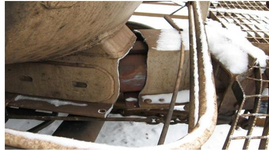
**Figure 1. Example of a cracked sill**
