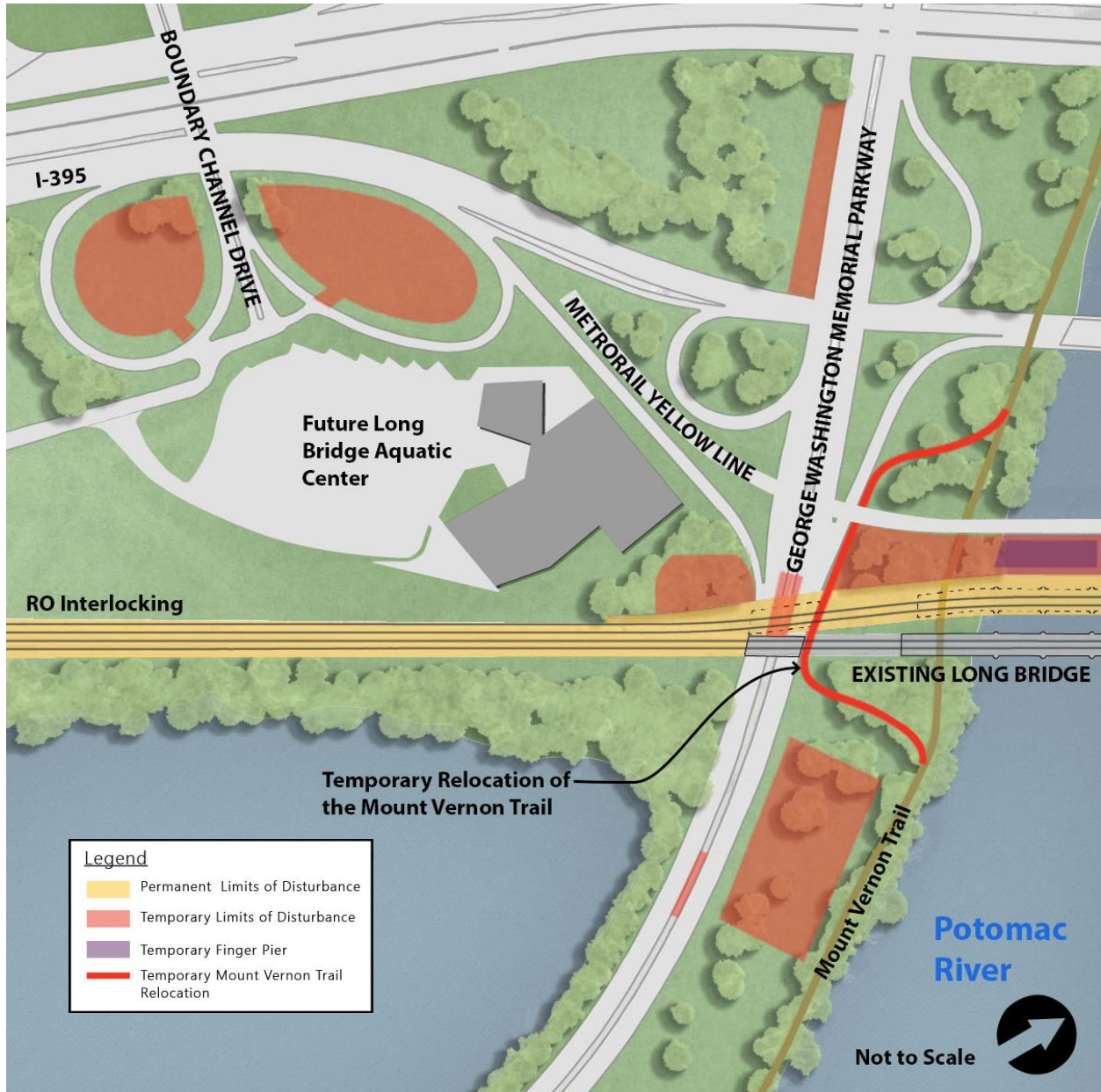
622 Figure 9-6 | Mount Vernon Trail Rerouting during Construction
