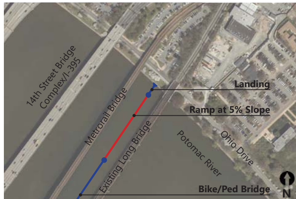
Landing with ramp over water
