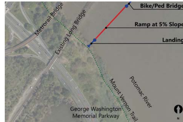
Landing with ramp over water
