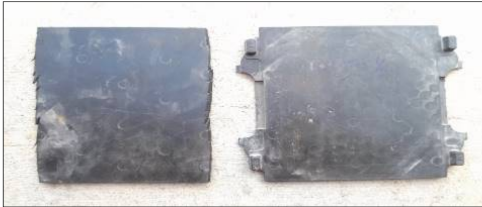
Figure 34. Cut Pad Simulating Deterioration (left) and Uncut Pad (right)
