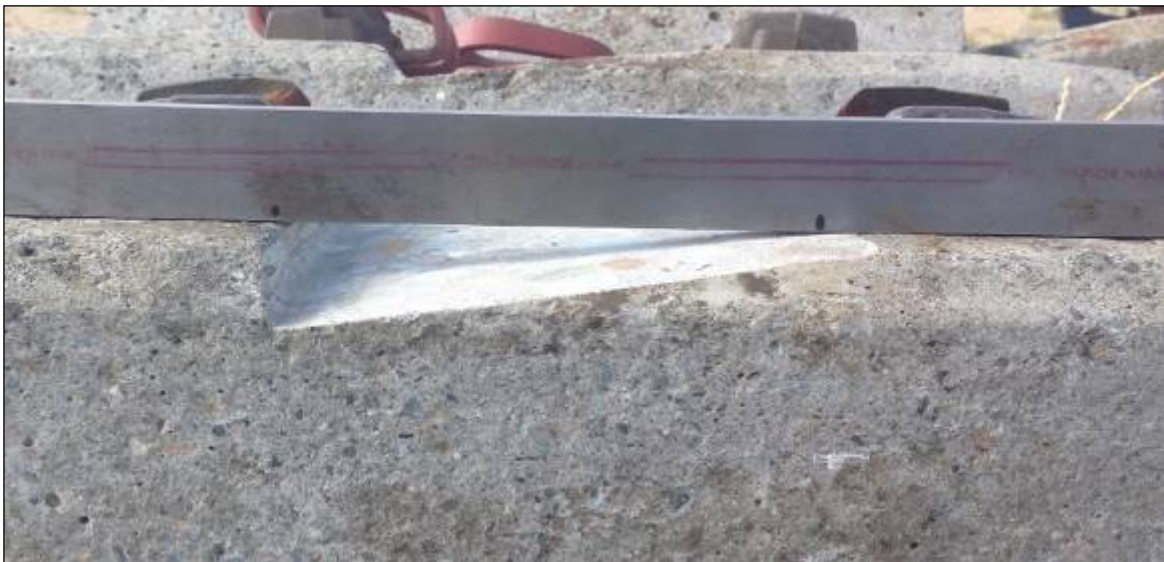
Figure 12. Example Showing Triangular RSD Depth Profile
