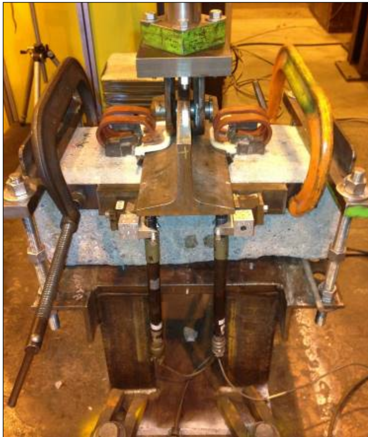
Figure 18. Vertical Rail Uplift Fixture
