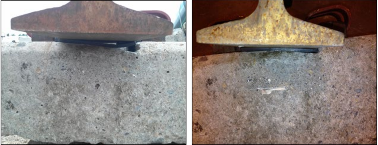
Figure 35. Using a New Rail Pad, Rail Before (left) and after (right) Lateral/Vertical Compliance Test
