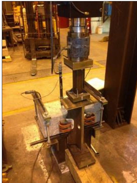
Figure 16. Rail Longitudinal Restraint Fixture
