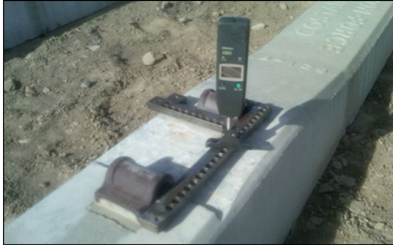
Figure 6. RSD Depth Measurement Gage used to Measure RSD of Ties Installed at FAST at 0 MGT and 375 MGT
