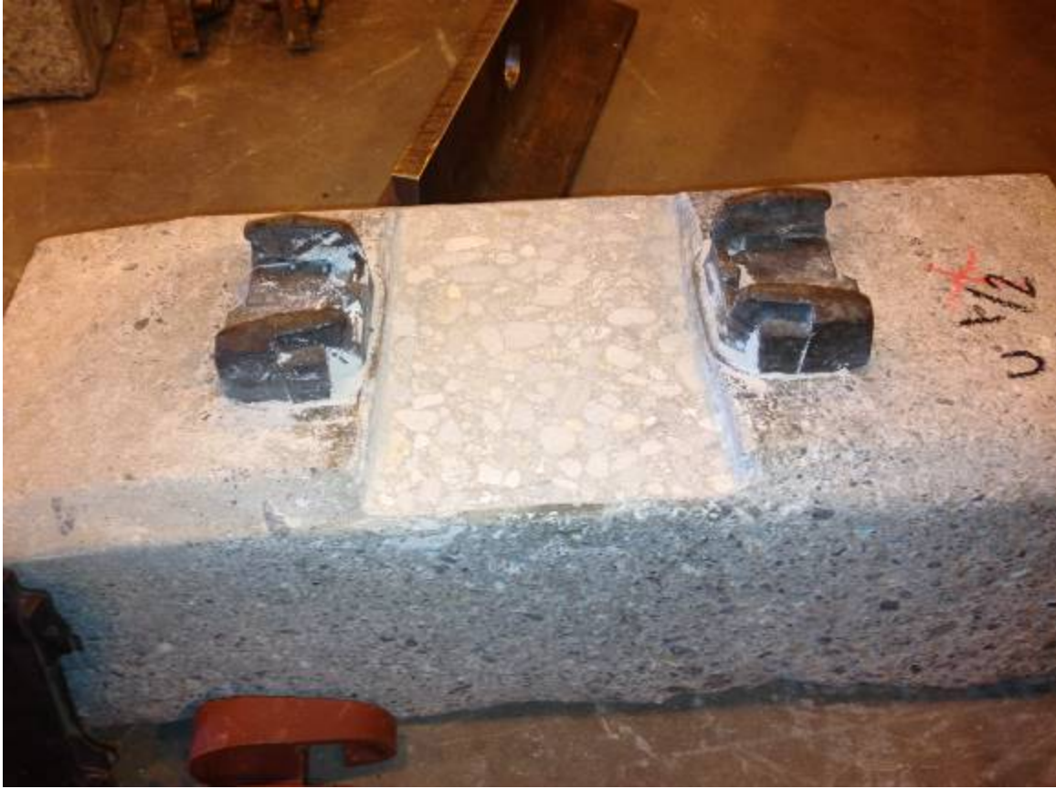
Figure 9. Example of Concrete Tie Section with Uniform RSD
