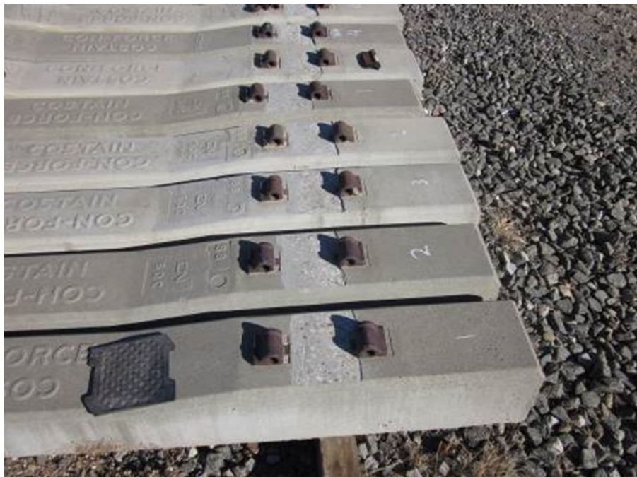
Figure 3. Rail Seats Ground to Simulate Triangular RSD before Installation at FAST (0 MGT)
