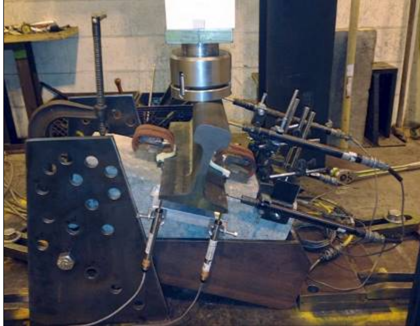
Figure 23. Lateral/Vertical Compliance Fixture
