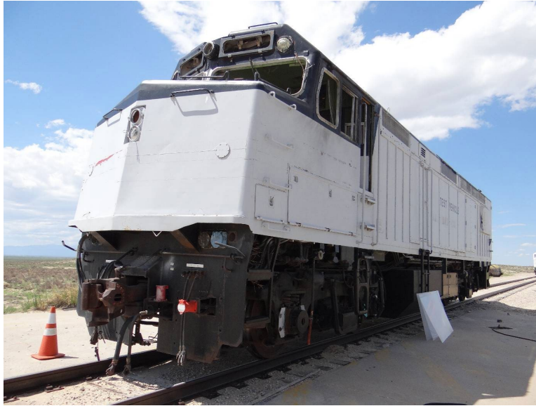
Figure 6. Un-modified (to S-580 requirements) EMD model F40-PH locomotive unit 202 at the TTC
