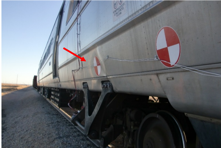
Figure 22. M1 side sill front-right truck connection (exterior view)
