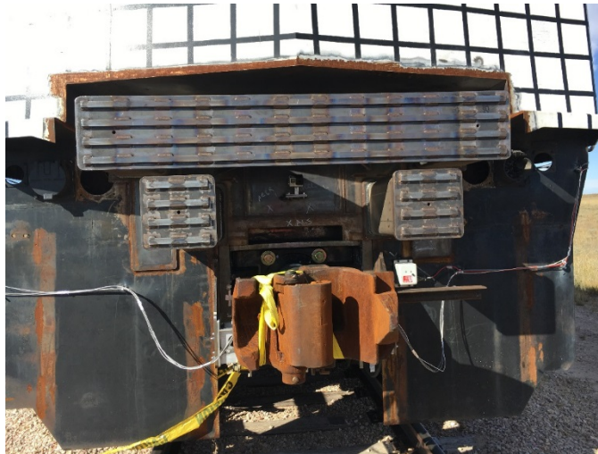
Figure 33. The DAC (top) and the PBC (bottom) comprise the locomotive CEM system
