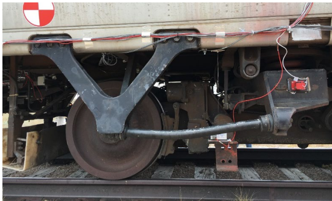
Figure 41. New M1 front left traction rod deformed again after 7mph test
