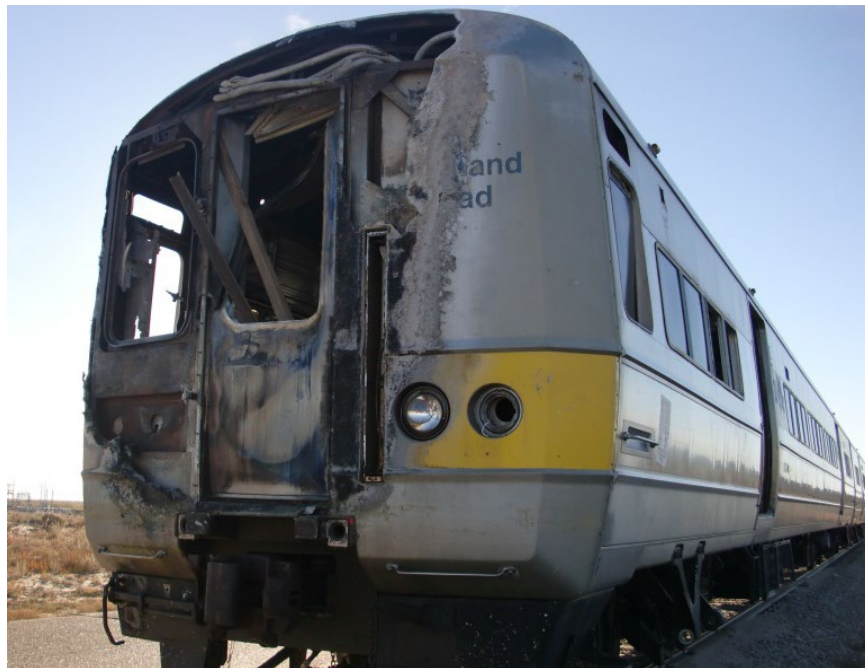
Figure 5. M1 cab car 9324 with some fire damage
