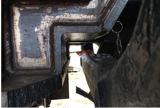
Figure 40. PBC flag and transom bar after 7 mph impact
