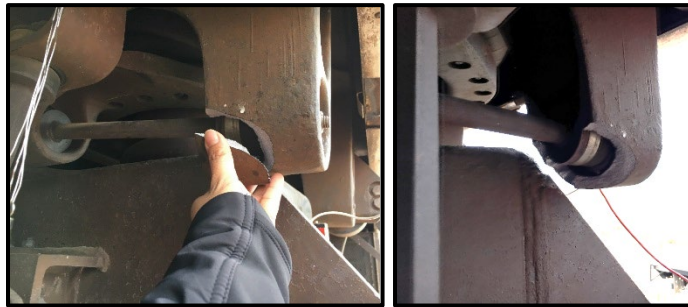
Figure 45. Piece broken off of M1 front-left truck, with piece held up to its former place (left)
