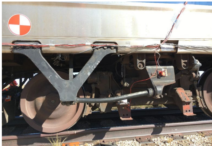
Figure 39. M1 front-left traction rod deformed after 6 mph test
