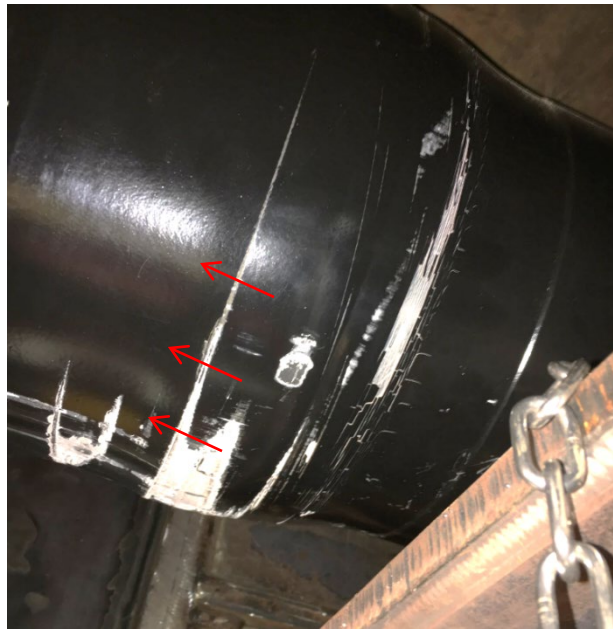
Figure 64. Cracked paint on the left side of the PBC deformation tube indicating tube crush
