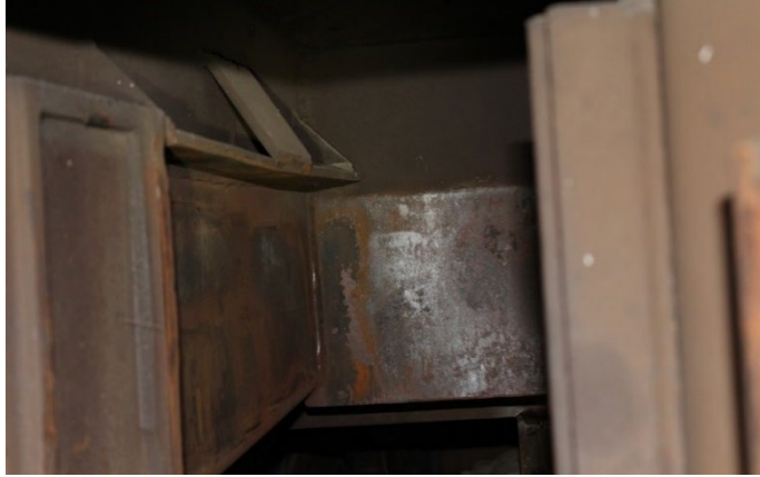
Figure 24. M1 interior draft pocket bent longitudinal member, right side
