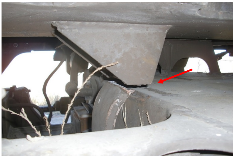
Figure 19. M1 front belt loop of front truck severed
