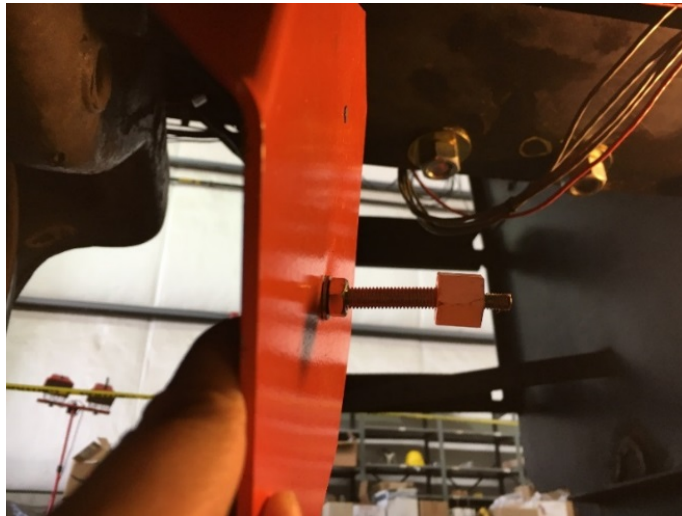
Figure 47. The PBC trigger indicator—an orange flag attached to the PBC by a bolt
