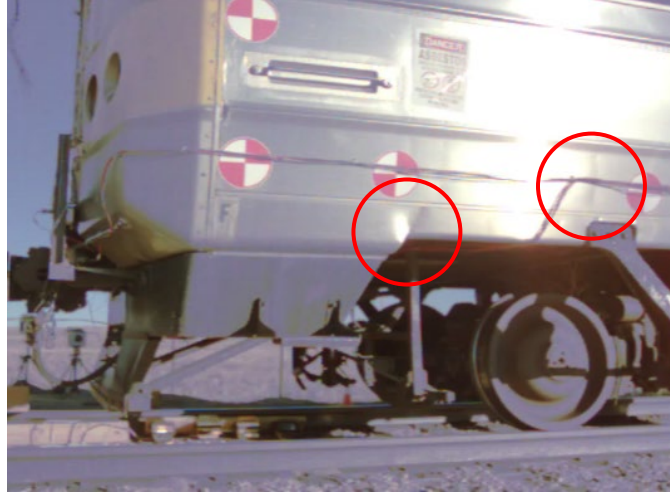
Figure 8. Dimpling of M1 shell at front-left side sill truck connection after 5.7 mph impact test
