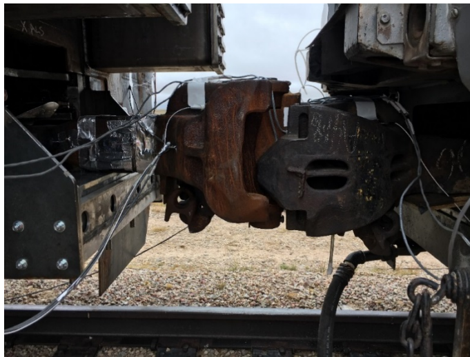
Figure 37. Vehicles did not couple in the 6 mph impact
