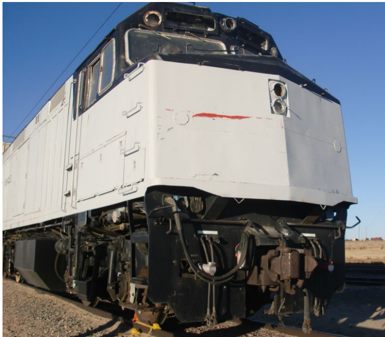
Figure 3. F40 Locomotive 202 used in the conventional coupling tests
