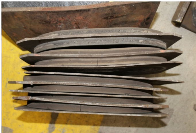
Figure 26. M1 bent buff plates
