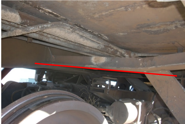
Figure 18. M1 underframe member bent near front truck connection, left side
