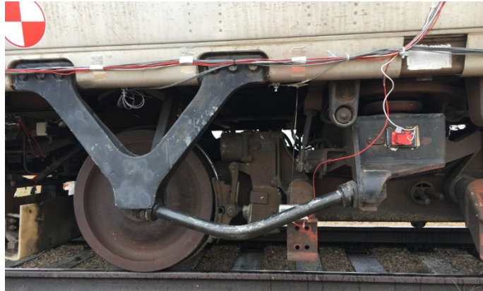
Figure 50. M1 front left traction rod deformed more after 9 mph test
