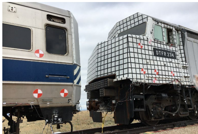
Figure 32. Pre-test photo of M1 cab car 8221 (left) and F40 Locomotive 234 (right) used in the CEM coupling tests
