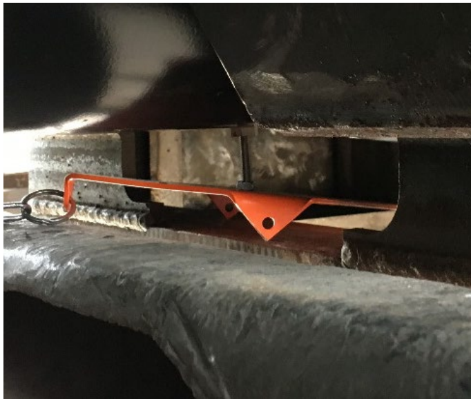
Figure 43. Close-up of the PBC flag and bolt after 8 mph impact
