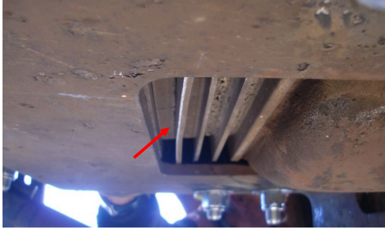
Figure 14. M1 bent buff plate in draft gear
