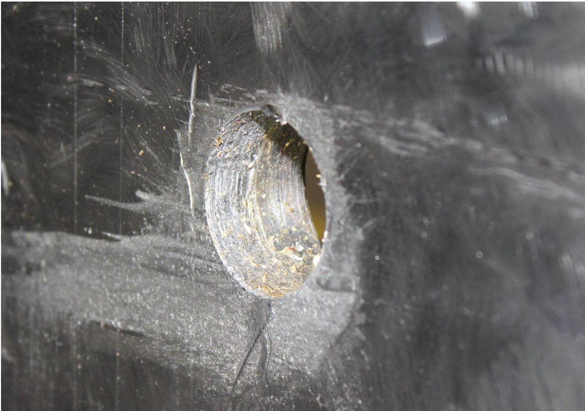
Figure 52. Surface damage at bolt hole (shear bolt 4, left rear middle position)
