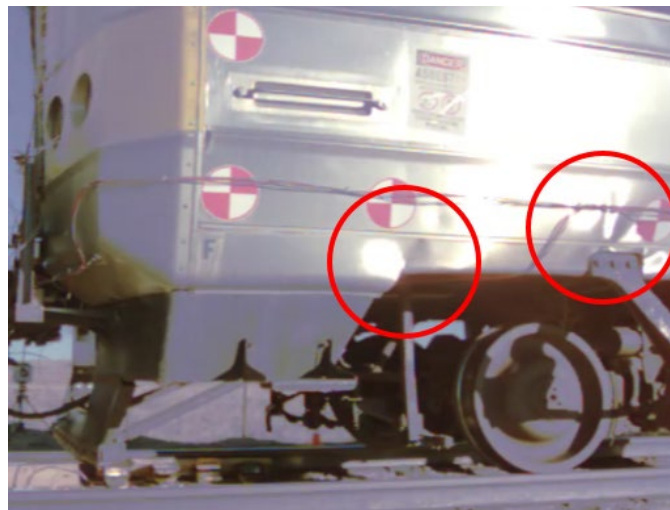
Figure 9. More pronounced dimpling of M1 shell at front-left side sill truck connection after 7.9 mph impact test
