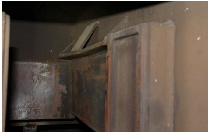
Figure 25. M1 interior draft pocket bent longitudinal member, left side
