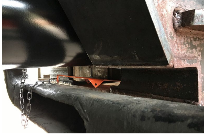
Figure 42. PBC flag and transom bar after 8 mph impact
