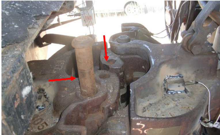
Figure 10. M1 coupler (left) hinge pin and locomotive coupler (right) knuckle damage
