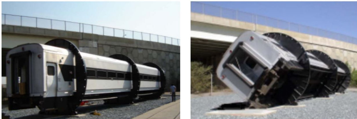
Figure 2.24 Emergency Evacuation Simulator ("Rollover Rig") (FRA, 2006)
