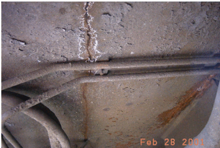
Fig. # 2 Crack in the connection plate along side draft gear pocket.
