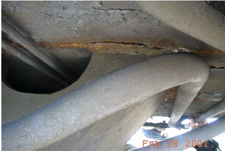
Fig. # 2 Crack in the connection plate along side draft gear pocket.
