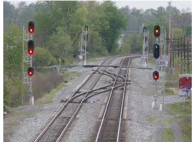
Example of Rail Interlocking
