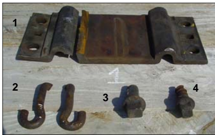
Figure 2. Component Failure under HAL Traffic (1) Pandrol 16-in. Rolled Steel Tie Plate (2) NorFast Rail Clip (3) LB&N Co. High Strength Screw Spike (4) No. 5760 Screw Spike
