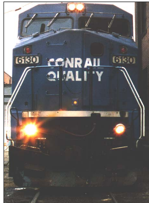
Figure 1. Alerting Light Triangle Using Auxiliary Crossing Lights
