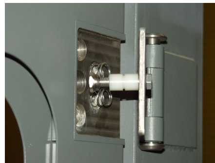
Figure 5. Exterior view of fastener bolts and hinge leaf released from the hinge support block
