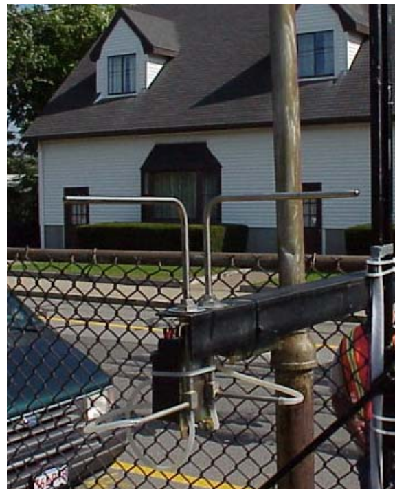
Figure 3. Pitot-static tubes mounted on stand for measuring airspeed.
