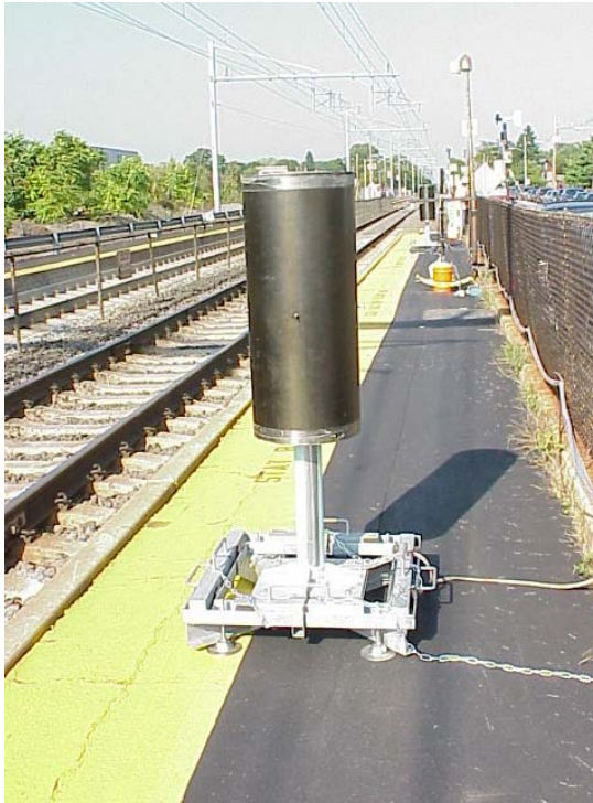
Figure 4. Circular cylindrical test dummy designed to measure resultant force applied to the cylinder.
