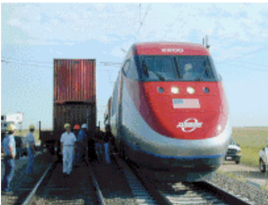
Figure 1. Test setup for high-speed train operating adjacent to container cars.
