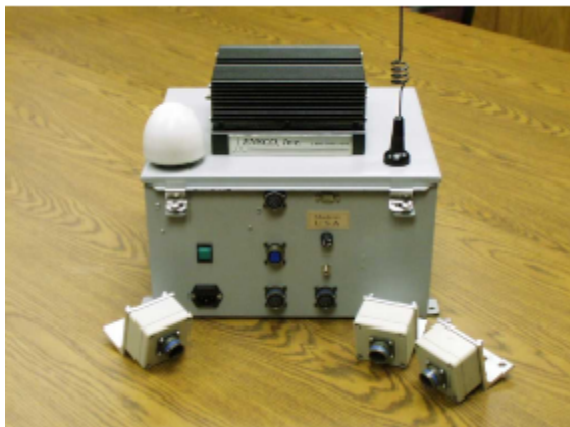
Figure 1. A light onboard platform with cellular/CDPD modem and accelerometers designed for passenger cars.
