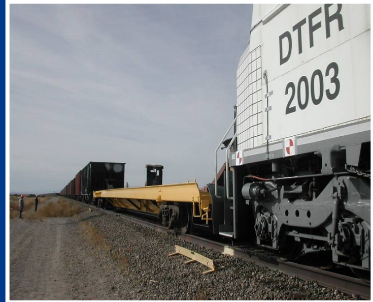
Height of flat car deck is below the base of the locomotive anticlimber
