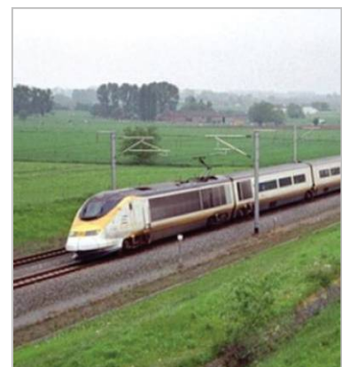
Figure 2-3 Example of an at-grade profile showing catenary wire system and vertical arms of the pantograph power pickups
