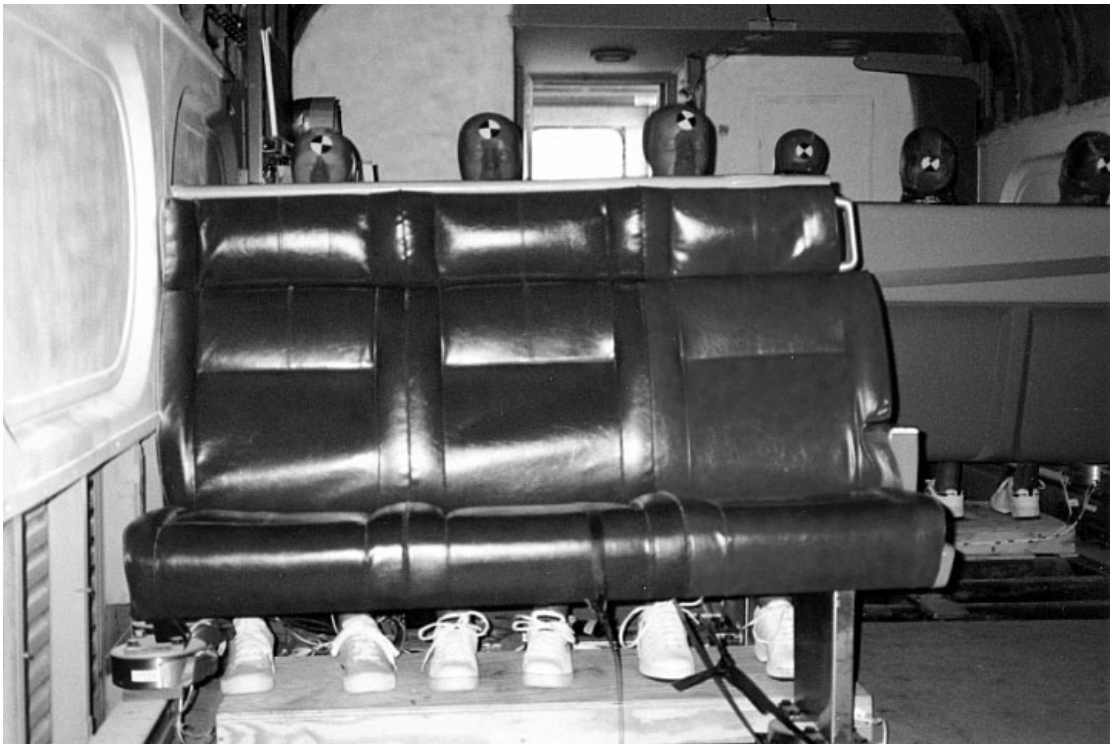
Figure 2. Pre-Test Photo of Experiment No. 1 – Row-to-Row Commuter Seats
