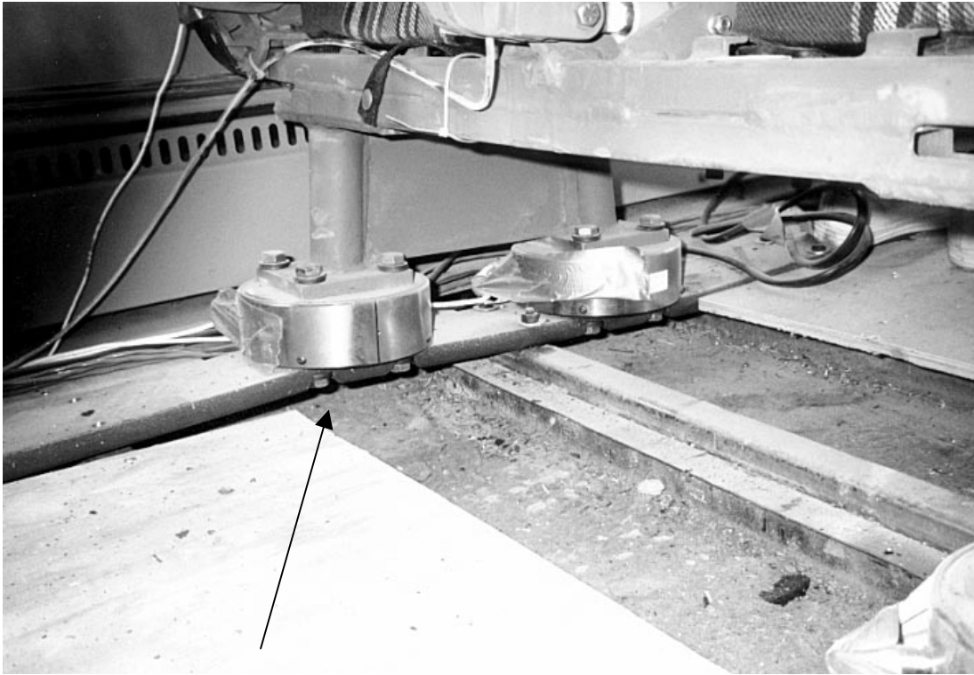
Figure 11. Experiment No. 2 – Metal Floor Attachment Bar Deformed Under Load
