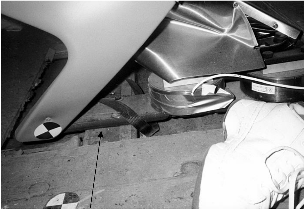
Figure 7. Experiment No. 1 – Front-Row Seat Pedestal Collapse and Seat Deformation
