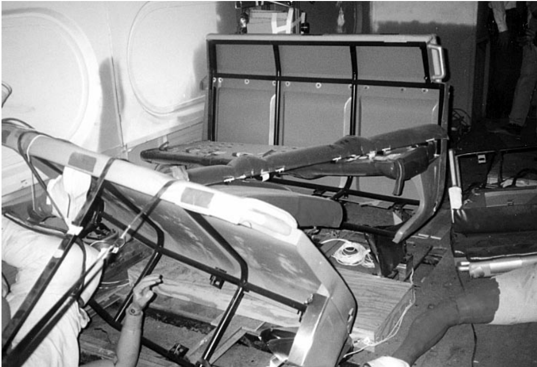
Figure 6. Experiment No. 1 – Loss of Passenger Compartmentalization
