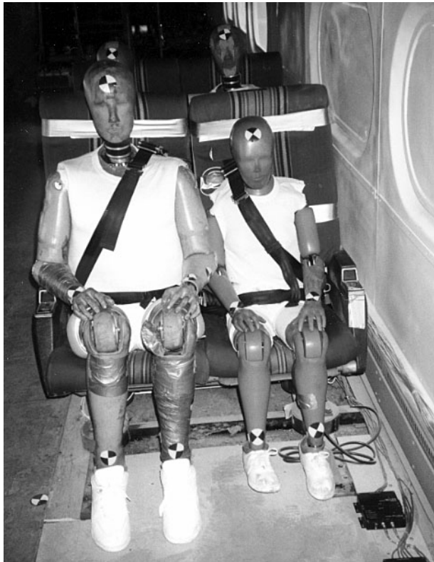
Figure 3. Pre-Test Photo of Experiment No. 2 – Row-to-Row Amtrak Seats with Restraints
