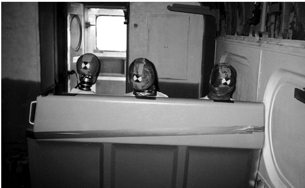
Figure 4. Pre-Test Photo of Experiment No. 3 – Rear-Facing Commuter Seat
