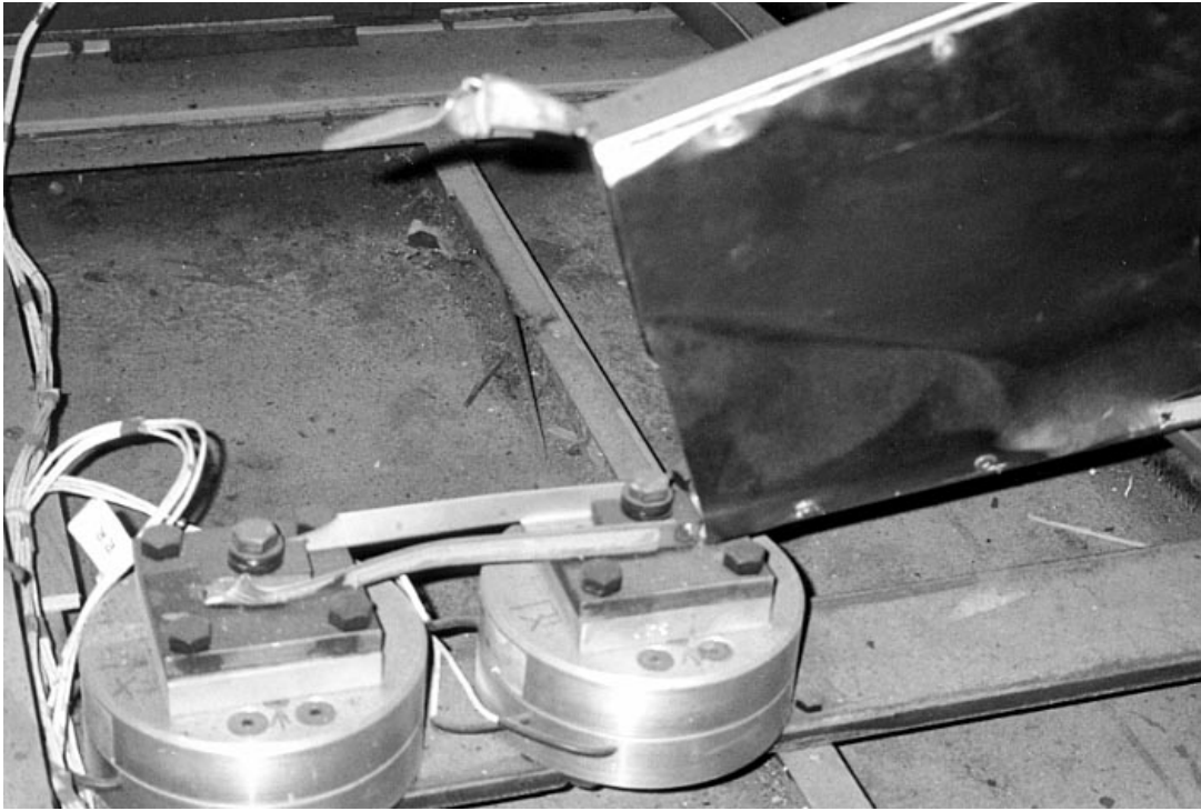
Figure 12. Experiment No. 3 – Seat Pedestal Sheared Near the Floor Attachment
