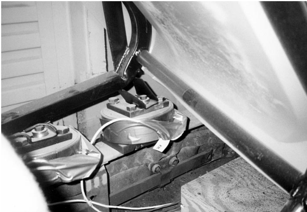
Figure 8. Experiment No. 1 – Front-Row Seat Frame Deformation and Weld Seam Failure
