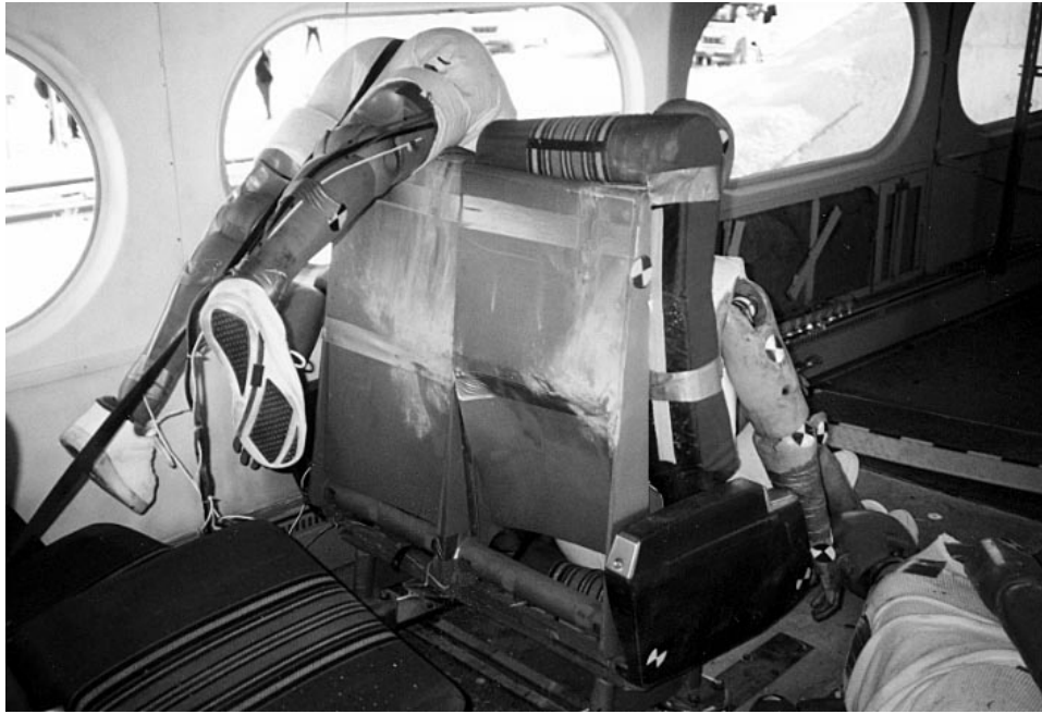
Figure 9. Experiment No. 2 – ATD Not Compartmentalized
