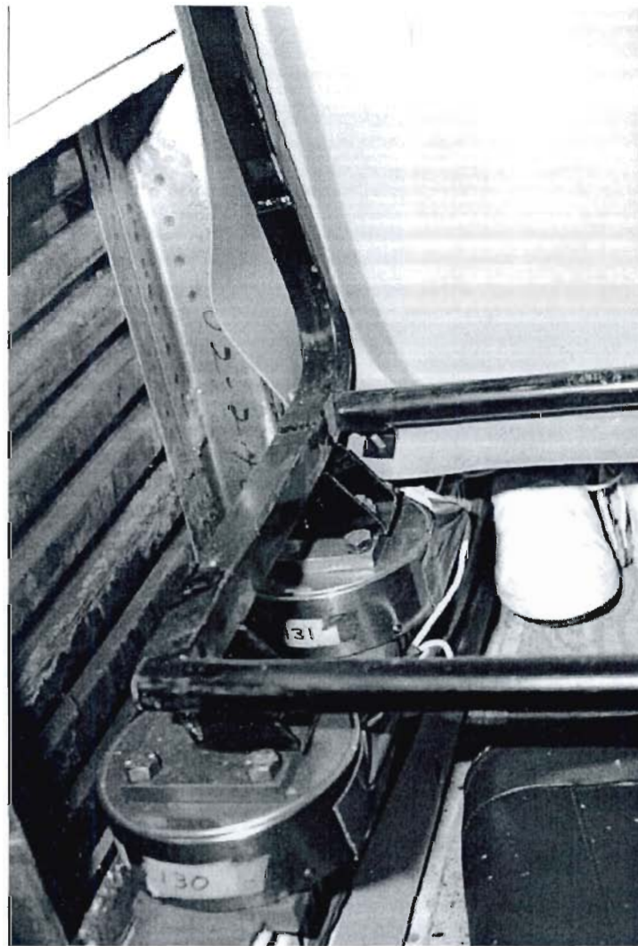
Figure 7. Experiment No. 2-1 – Post-Test Photograph of Side Wall Frame and Shroud Deformation
