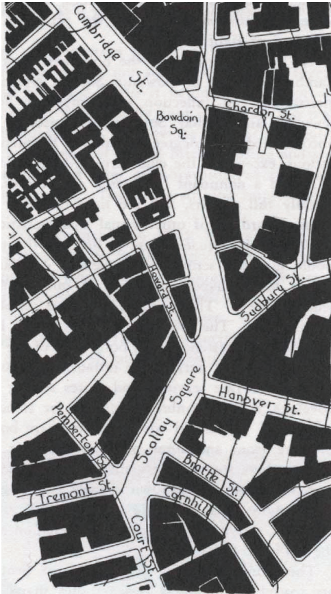
Above: Drawing of Scollay Square from The Image of the City . Kevin Lynch. MIT Press. 1960. Drawing of buildings as figure and streets/squares as ground. Figure-ground drawings can help designers understand the urban fabric as a composition of positive and negative spaces represented by dark and light.
