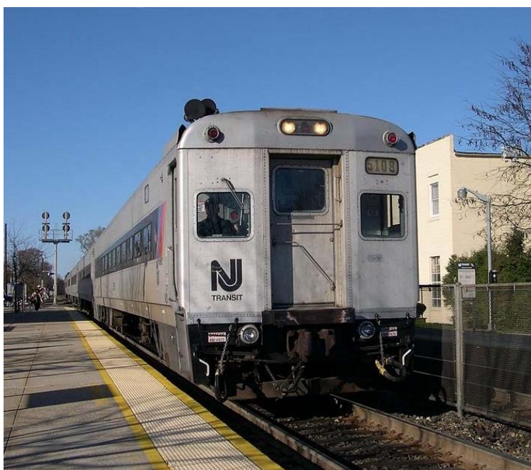
Figure 1. An Example of a Cab Car in which the Operator is Positioned Immediately Adjacent to the Vehicle End
