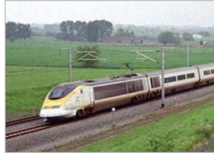
Figure 2-3 Example of an at-grade profile showing contact wire system and vertical arms of the pantograph power pickups
